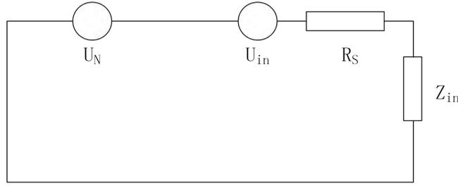
Figure 1 – Equivalent circuit diagram of inductive coupling model.
