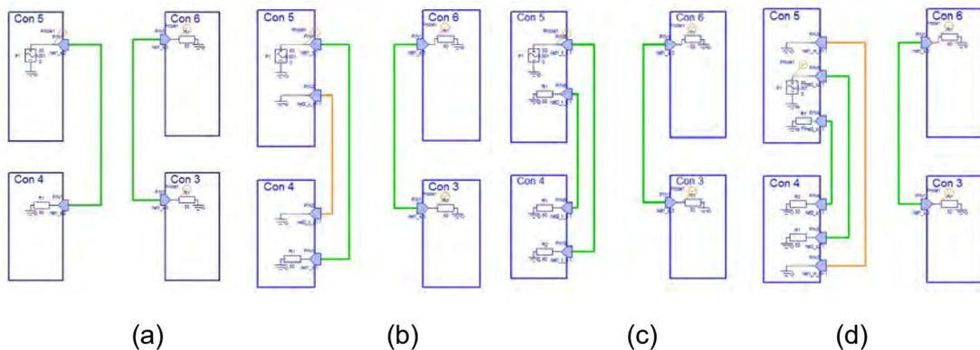
Figure 3 – Cable simulation circuit: (a) single core single core; (b) Coaxial line - Single core; (c) Twisted pair - Single core; (d) Shielded twisted pair - Single core.
