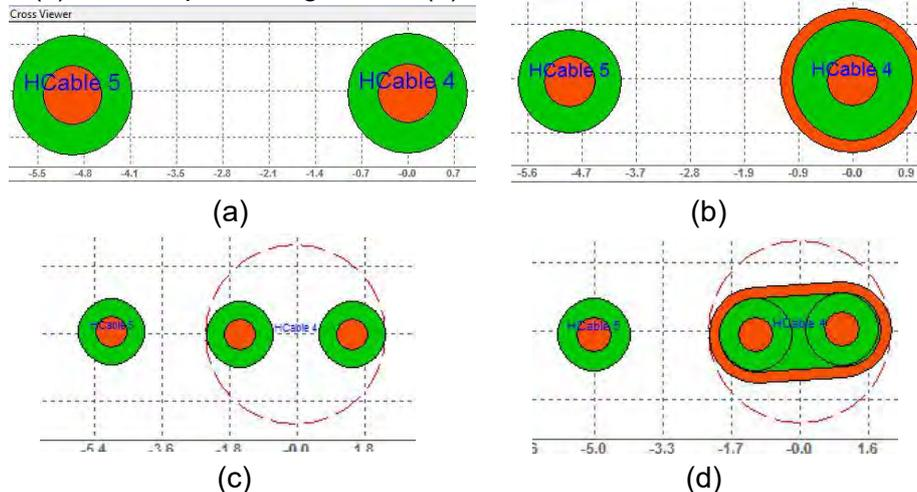
Figure 4 – Simulation cable setting: (a) single core wire; (b) Shielded single core wire; (c) Twisted wire; (d) Shielded twisted wire.
