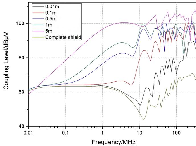
Figure 10 – The relationship between crosstalk level and the length of stripped shielding layer of single core shielded cable.
