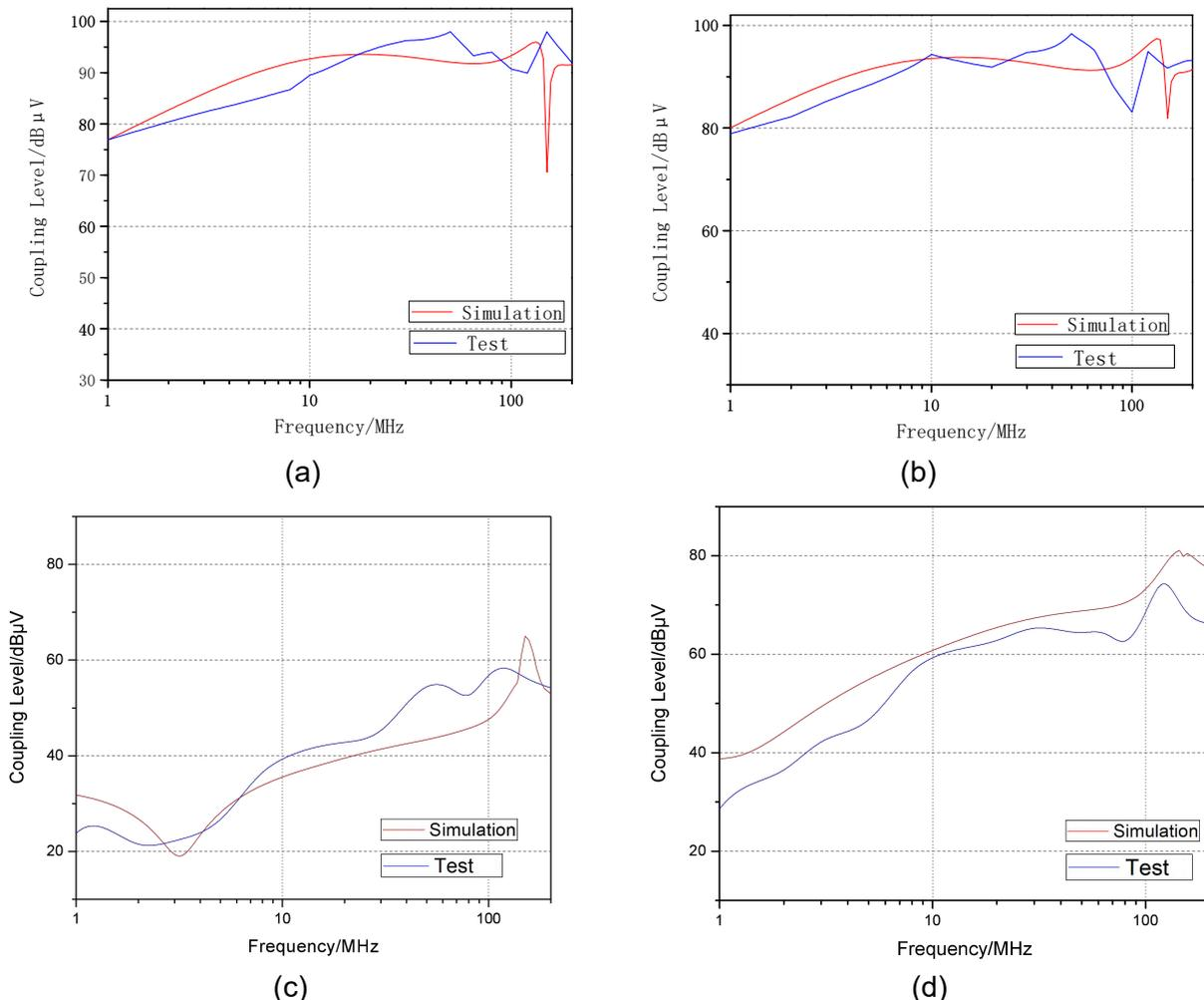
Figure 7 – Actual test verification results: (a) single core wire; (b) Shielded single core wire; (c) Twisted wire; (d) Shielded twisted wire.
