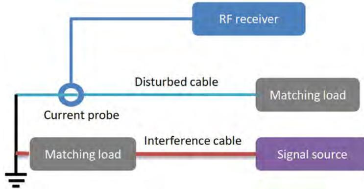
Figure 6 – Crosstalk Test diagram
