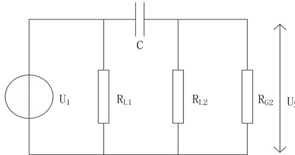
Figure 2 – Equivalent circuit diagram of capacitive coupling model.
