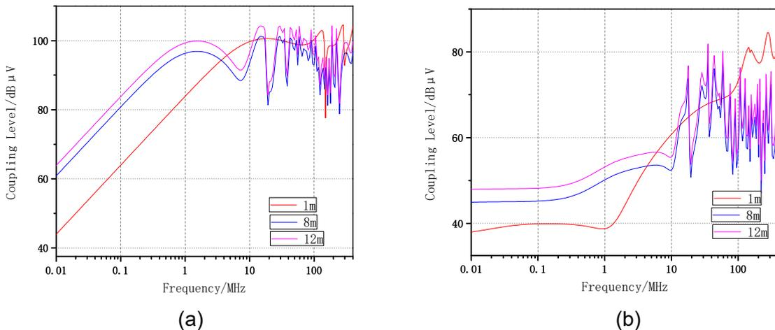
Figure 9 – Simulation results of conductive coupling of cables with different lengths:
