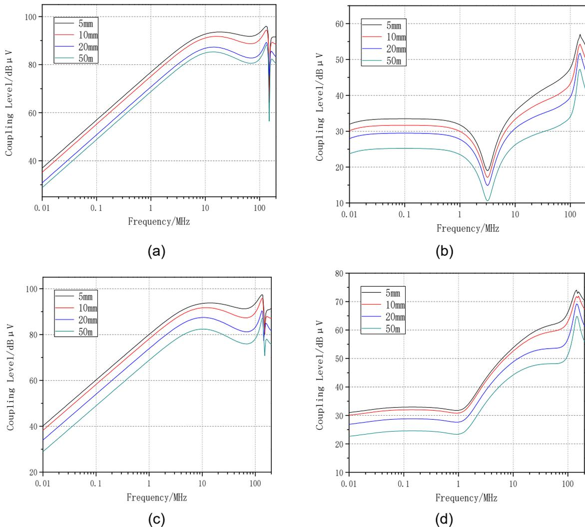
Figure 5 – Crosstalk characteristics simulation results: (a) single core wire; (b) Shielded single core Wire; (c) Twisted wire; (d) Shielded twisted wire.
