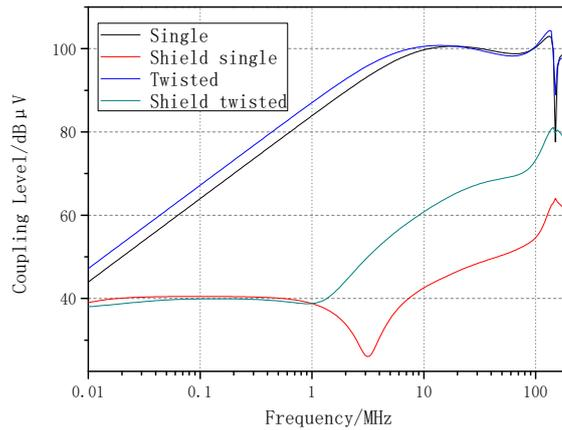
Figure 8 – Crosstalk coupling of different types of cables.
