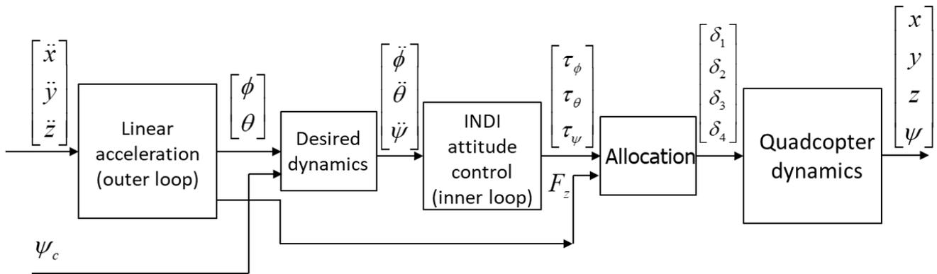
Figure 2 - Block diagram of INDI with two-time scale separation
