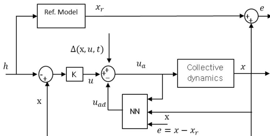
Figure 1 - Augmented adaptive decentralized formation control.
