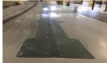
Stiffener installed in the tool aiming at deforming it at the required geometry (kink angles)
