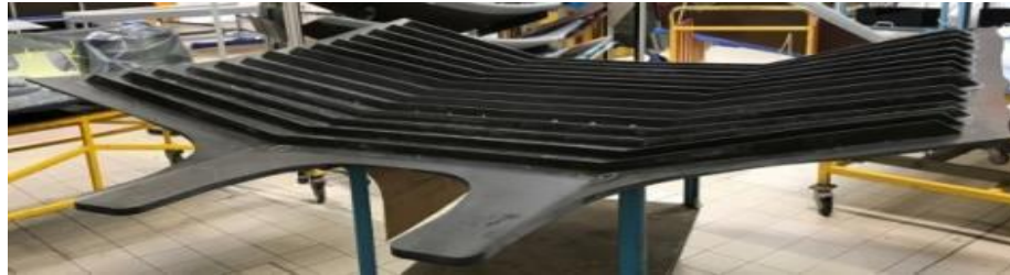
Stiffener installed in the tool aiming at deforming it at the required geometry (kink angles)
