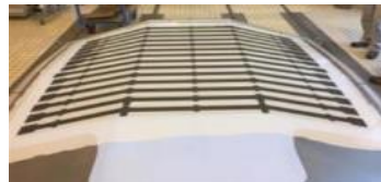
Stiffeners installed in the curing tool (co-bonding of the skin with the stiffeners)
