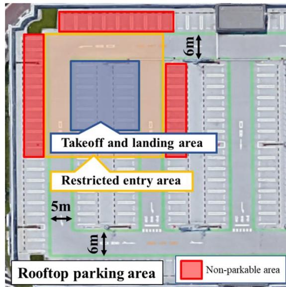
Figure 8. Assumed results of takeoff/landing site installation
