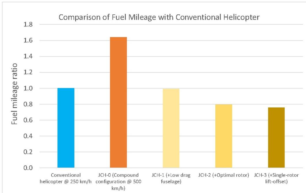
Figure 20 – Comparison of fuel mileage of compound helicopter with a conventional helicopter [19].
