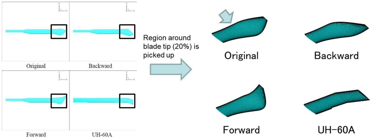
Figure 7 – Blade tip portion models [13].
