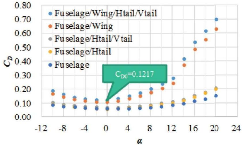
Figure 18 – Drag coefficient of the compound helicopter model with various configurations [16].
