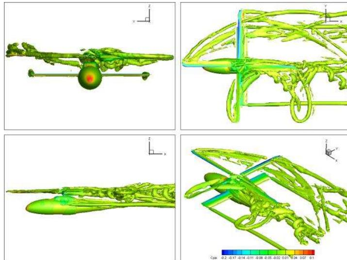
Figure 9 – Visualization of the flow field around the main rotor and a winged fuselage [9].
