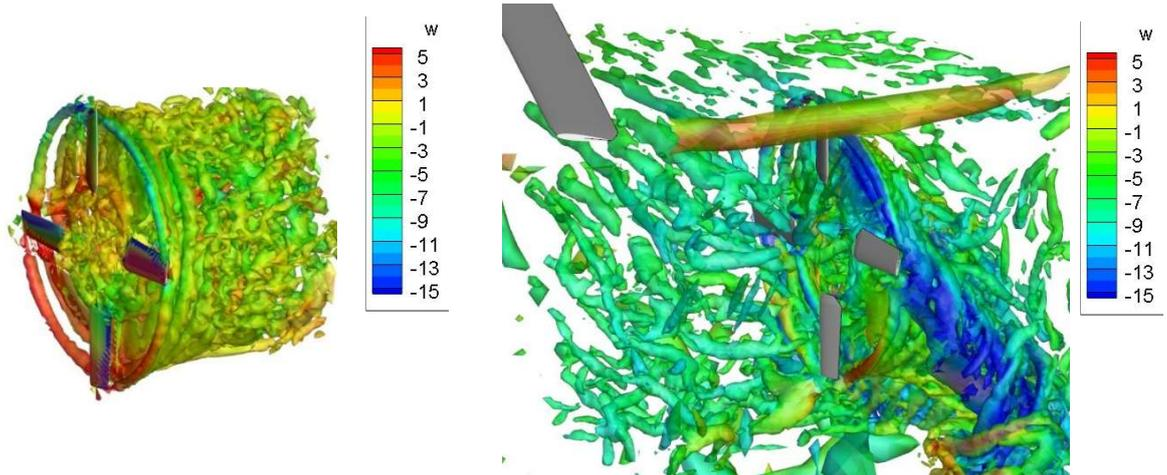
Figure 15 – Flow field around an isolated side propeller (left) and a side propeller with the main rotor (right).
