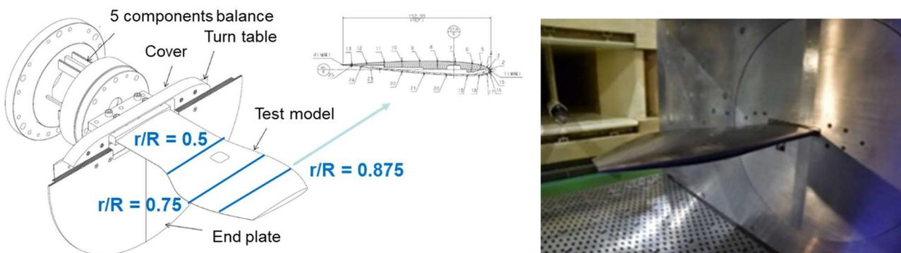
Figure 8 – Transonic wind-tunnel testing of the blade tip portions [13].
