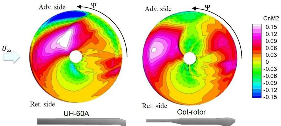
Figure 12 – Normal loading ( $C_n M^2$ ) distribution on the rotor discs at  $\mu = 0.7$  [10].
