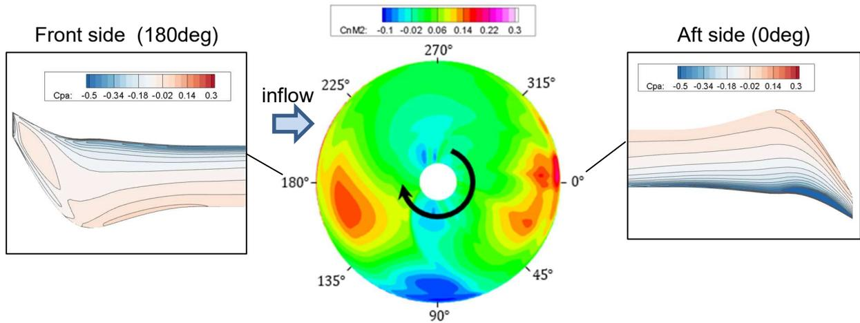
Figure 6 - Normalized lift distribution on the rotor disk with pressure distribution at front/aft positions (Forward swept blade)
