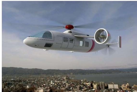
Figure 1 – A conceptual design of a high-speed compound helicopter.
