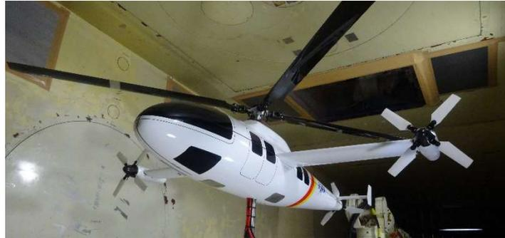
Figure 13 – Model compound helicopter with main rotor and side propellers.
