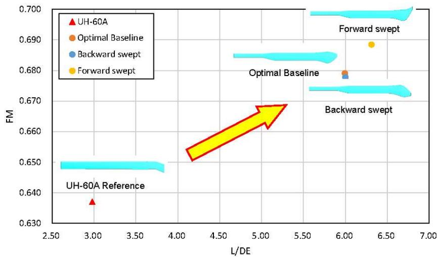
Figure 3 – Optimal rotor blade design for flight at  $\mu=0.7$ .
