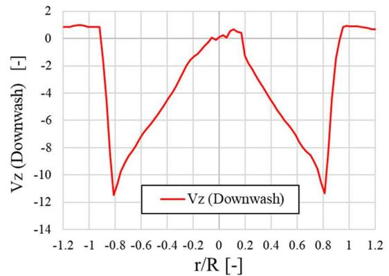
Figure 14 – Downwash from the main rotor at the position of the side rotor in hover [14].
