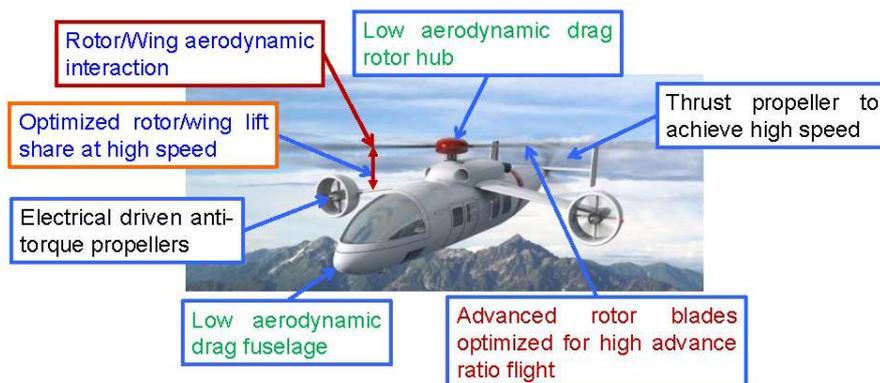
Figure 2 – Key technology issues to realize an efficient high-speed compound helicopter.
