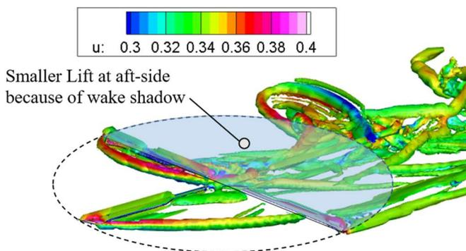
Figure 4 – Illustration of the relationship between wake shadow and front/aft moment balance
