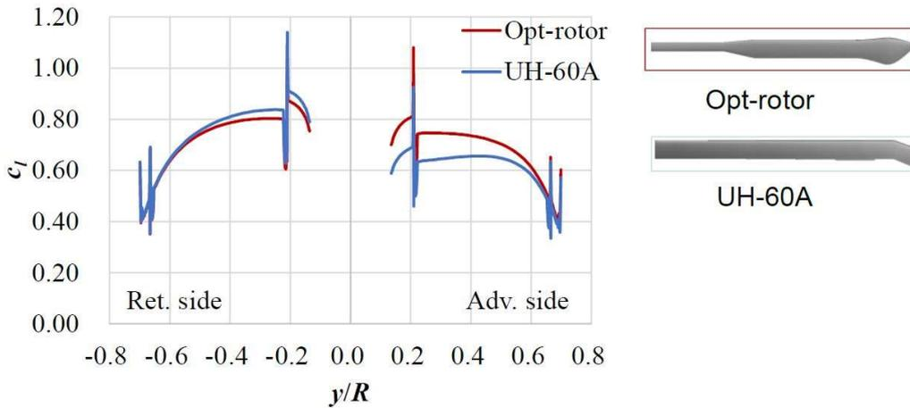
Figure 11 – Lift distributions on the wing for the optimal and UH-60A rotors [10].
