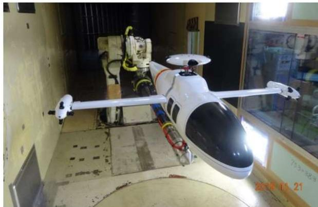
Figure 17 – Wind-tunnel testing of the fuselage of the compound helicopter model [16].
