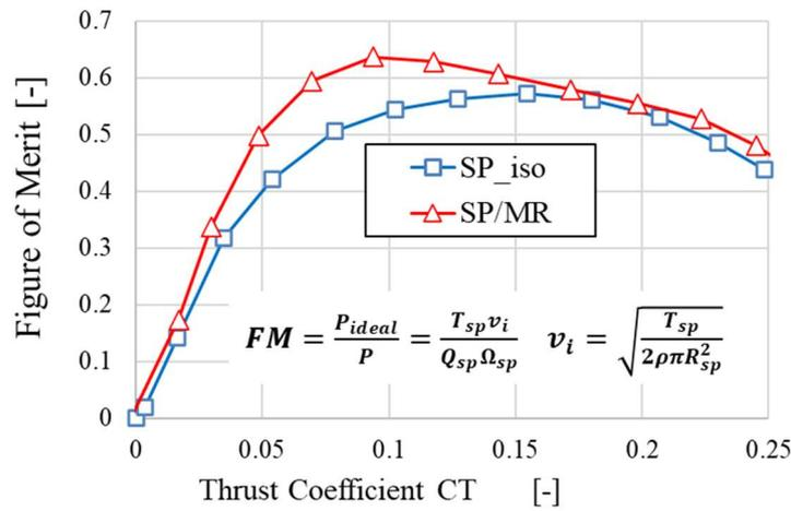
Figure 16 – Thrust and figure of merit of the side propeller [14].
