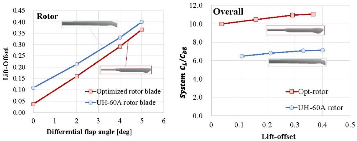
Figure 10 – Single-rotor lift-offset vs differential flap angle and improvement of system lift-drag ratio [10].
