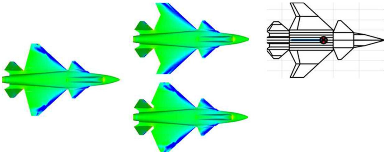
Figure 6 – CFD results used for configuration choice, Euler and panel code.
