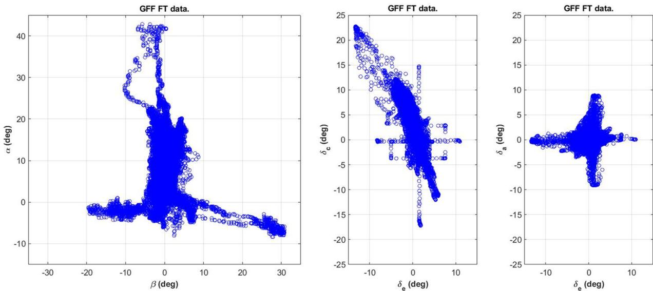
Figure 12 – Flight test envelop and configuration for the original wing configuration.
