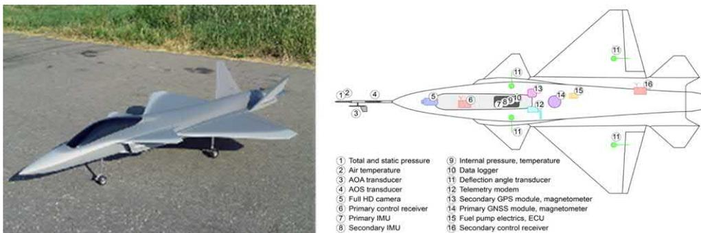
Figure 2 – The GFF aircraft and its data acquisition system.
