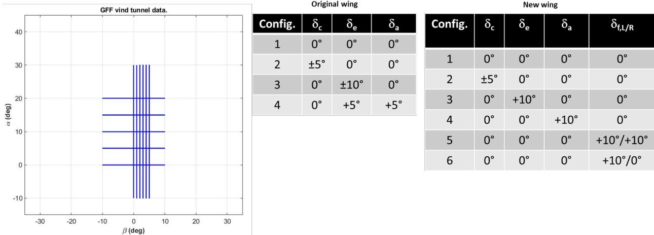
Figure 9 – Wind tunnel envelop, where the deflection of the the entire trailing edge on the Left/Right side for the new wing is denoted  $\delta_{f,L/R}$ .
