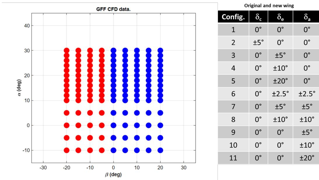
Figure 8 – CFD envelop and control surface configurations.
