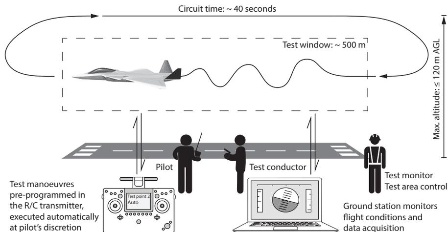
Figure 3 – Cost-efficient flight testing within VLOS using both manual piloting and automation.
