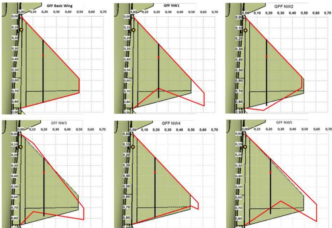
Figure 4 – Wing planform of the original aircraft and the five different concepts.
