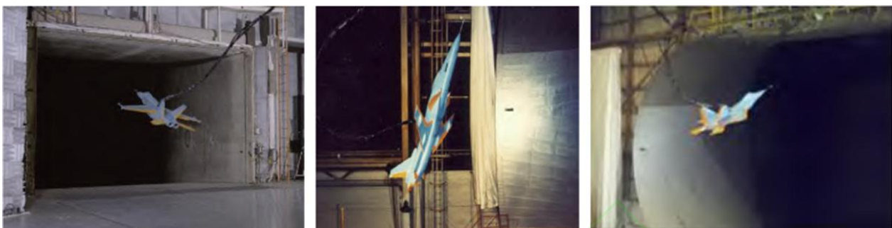
Figure 1 – Free-flight test in wind tunnel of NASA Langley Research Center
