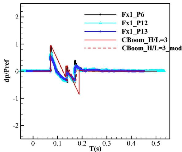
Figure 4 Comparison of over-pressure signatures for ground sonic boom (Ma=1.23)
