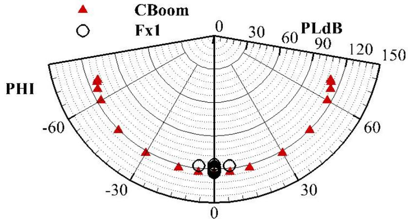
Figure5 Comparison of loudness levels for ground sonic boom signatures (Ma=1.23)
