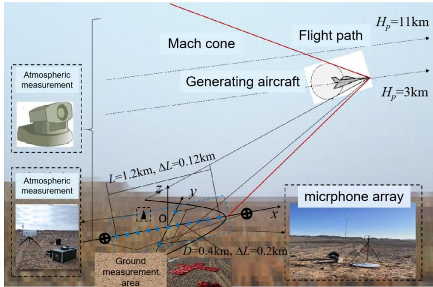
Figure 1 In-flight test method
