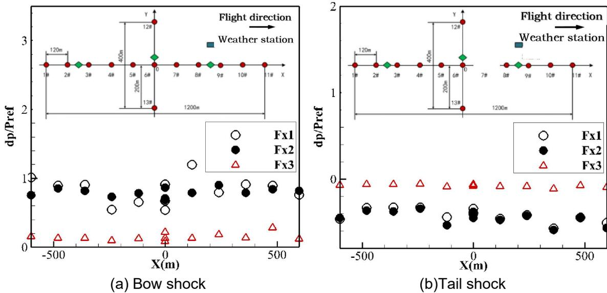
Figure 2 Peak over-pressure of the measured sonic boom signature
