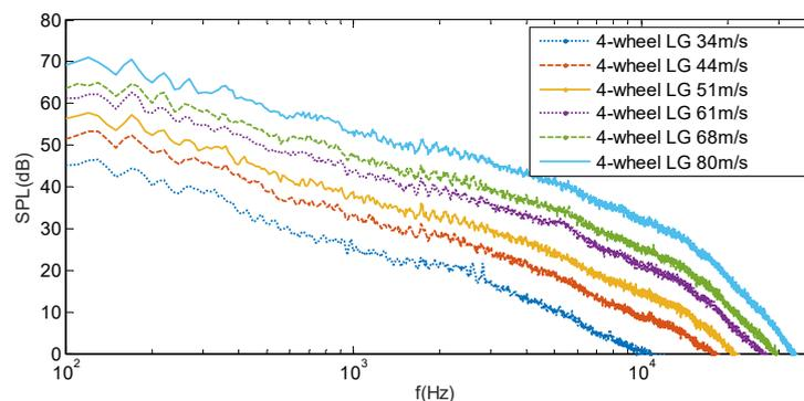
Fig.20 Landing gear noise spectrum curve under different wind speed
