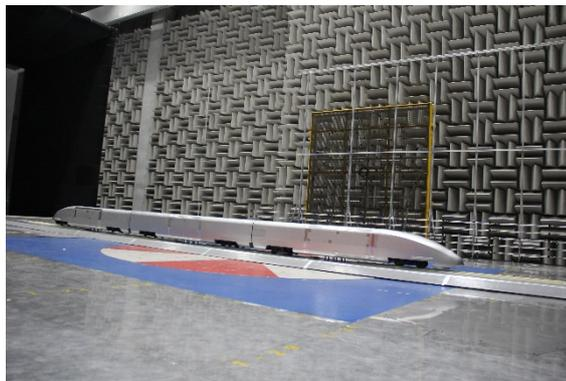
Fig 22 High speed train noise test in FL-10 WT
