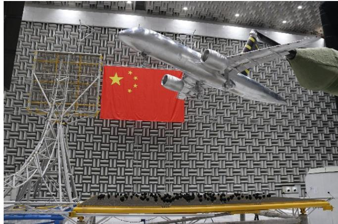
Fig.15 Airframe noise test in FL-10 WT
