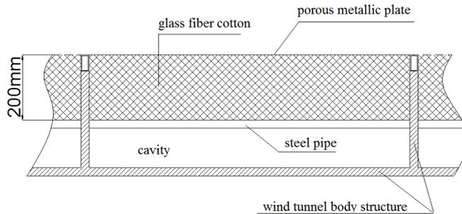
Fig.5 Outside acoustic treatment of wind tunnel
