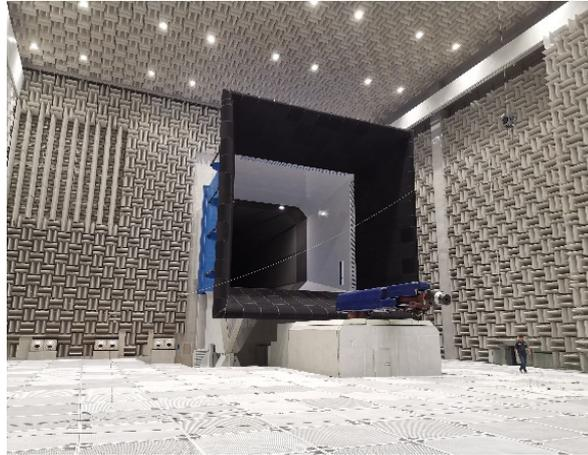
Fig.2 Anechoic chamber of FL-10 wind tunnel
