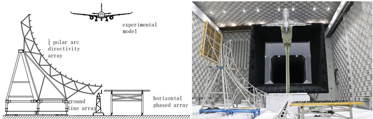
Fig 8 Array lay out for the scaled a/c model noise experiment
