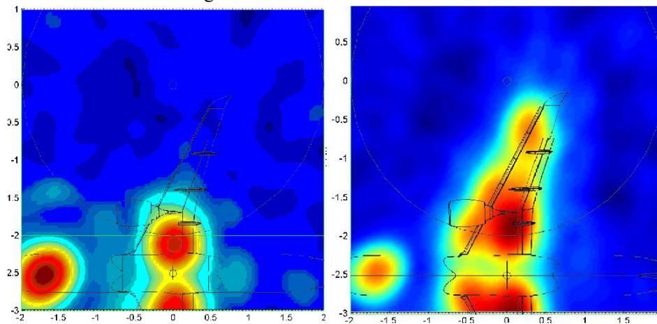
(a) Landing gear noise source localization result (b) Landing gear and high lift device noise source localization result
