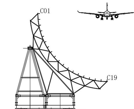
Fig 12 1/4 polar arc array (front view)
