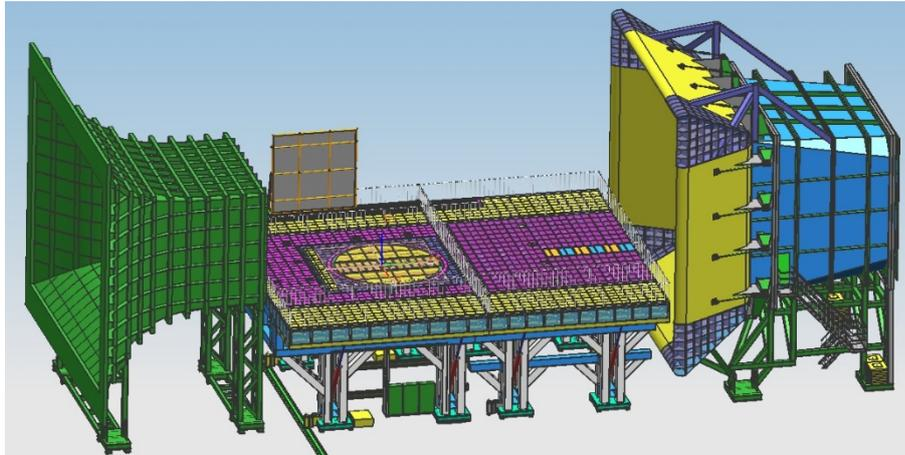
Fig 21 High lift device noise measurement platform
