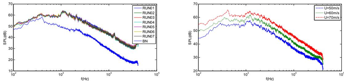
(a) Spectrum repeatability of takeoff configuration (b) Influence of wind speed on approach configuration spectrum
