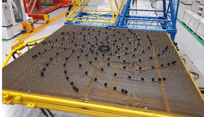
Fig 11 Vertical phased array (ground commissioning)
