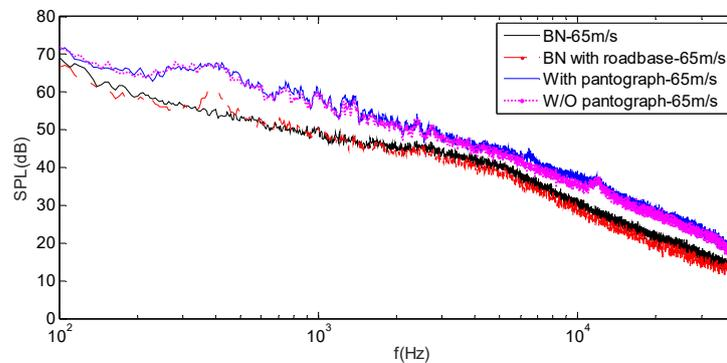
Fig.23 Noise spectrum w/o pantograph at 65m/s
