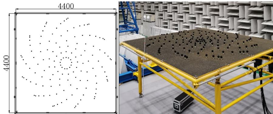
Fig 10 Sensor distribution of the array and real subject
