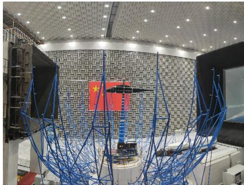
Fig 24 Helicopter noise experiment in FL-10 wind tunnel
