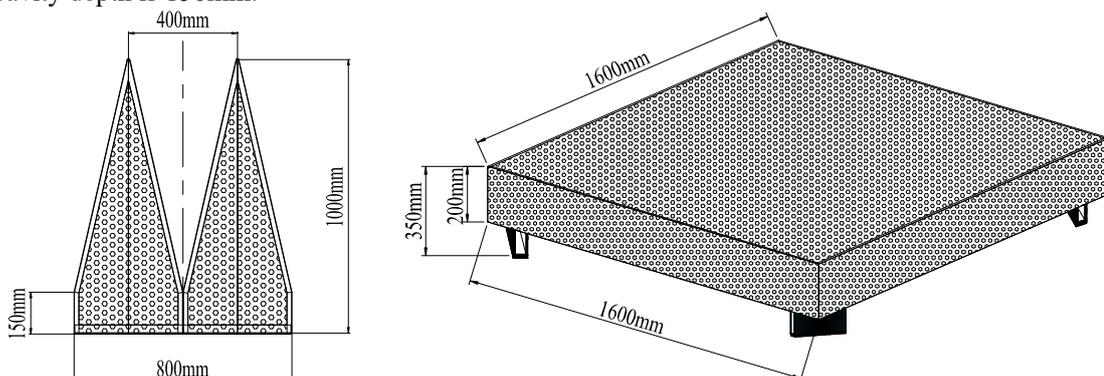
Fig.3 Sketch of acoustic wedge
