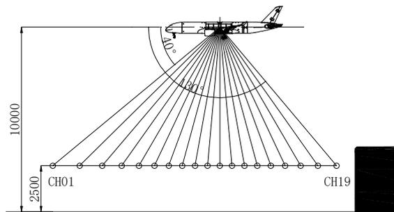
Fig 9 Sensor distribution on the ground line array
