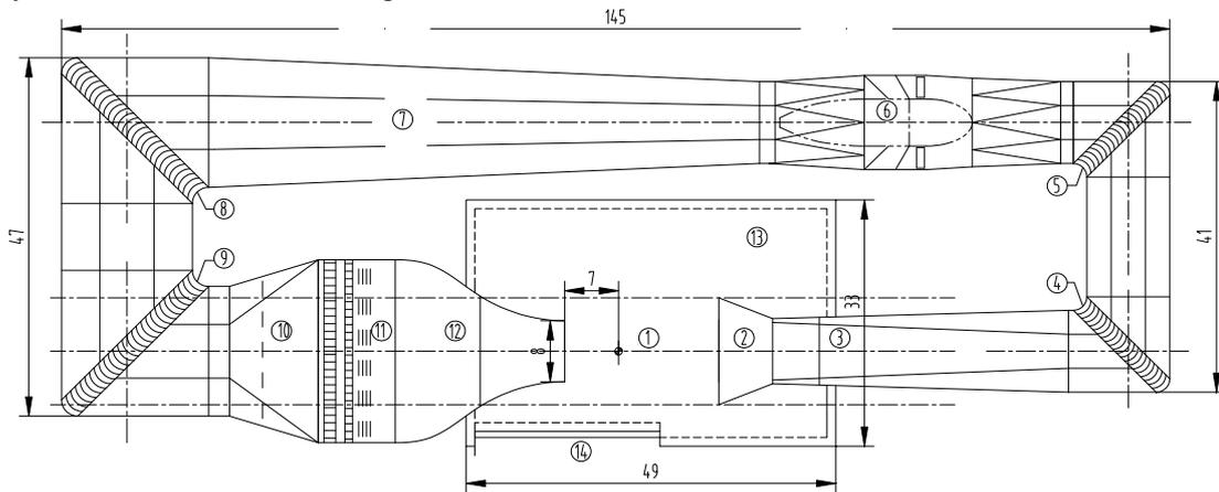
1.-open jet test section; 2.-collector; 3.first diffusor section; 4.-first corner; 5.-second corner; 6.-pove section 7.-second diffusor section; 8.-third corner; 9.-fourth corner; 10.-large angle diffusor section; 11.-stablizing section; 12.-contraction section; 13.-anechoic chamber; 14.-sound insulation
