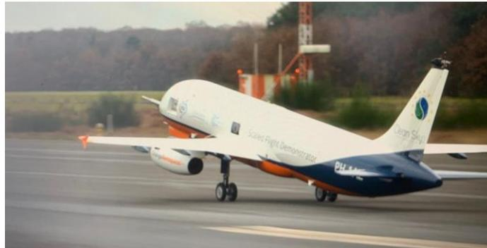
Figure 7 : Rotation Manoeuvres made with the SFD during the Taxi tests
