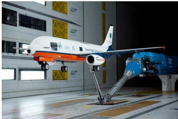
Figure 4 : Wind Tunnel Test installation of the SFD (DNW)
