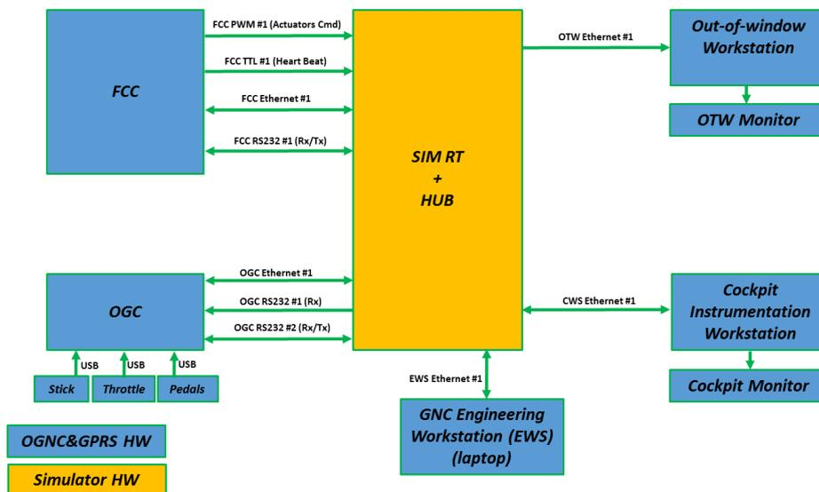
Figure 10 : Overall architecture of the Hardware-in-the-Loop test environment
