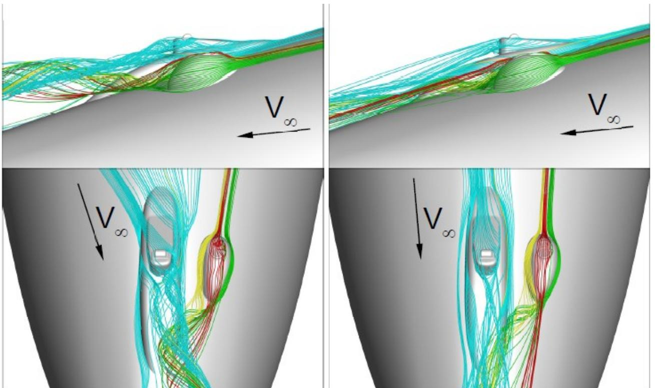
Figure 3 – Indicative flow topologies showing the radome wake characteristics with positive AoS
