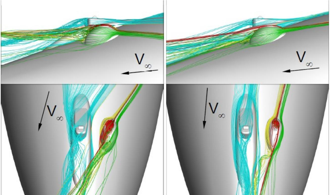
Figure 2 – Indicative flow topologies showing the radome wake characteristics with negative AoS
