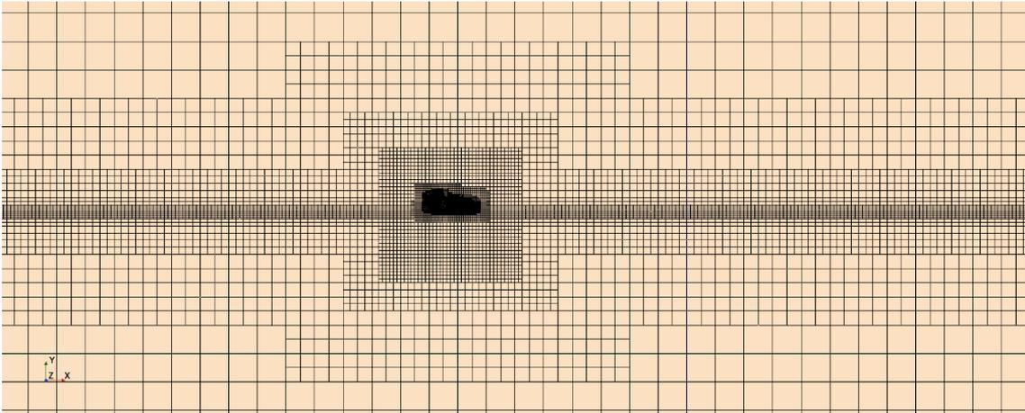
Figure 3 – Domain shape and mesh. It is visible a denser mesh at the fluid interface and in two size box centred in the hull.
