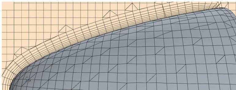
Figure 4 – Prism Layers
