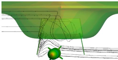
Figure 25 Streamlines around missile t=0.42s  $\beta=3^\circ$
