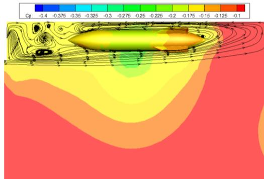
Figure 14 Streamlines around missile  $\alpha=2^\circ$   $t=0$ s
