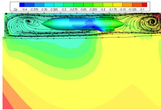
Figure 16 Streamlines around missile  $\alpha=-2^\circ$   $t=0s$
