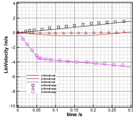
Figure 6 Variation of line velocity of missile with time
