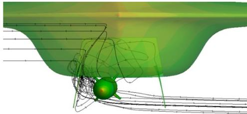
Figure 24 Streamlines around missile t=0.34s  $\beta=3^\circ$
