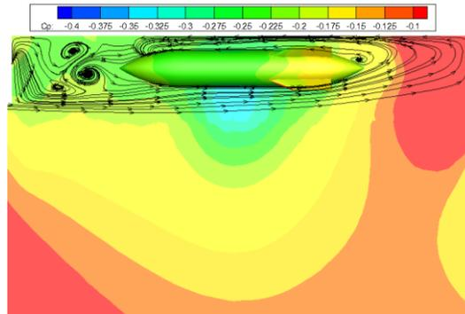
Figure 13 Streamlines around missile  $\alpha=0^\circ$   $t=0$ s
