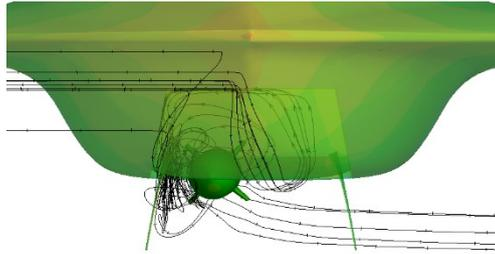
Figure 23 Streamlines around missile t=0.26s  $\beta=3^\circ$
