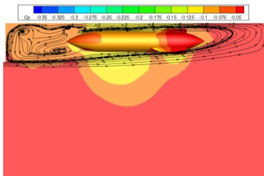
Figure 15 Streamlines around missile  $\alpha=6^\circ$   $t=0$ s
