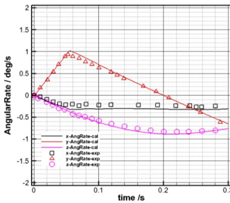
Figure 7 Variation of angle rate of missile with time
