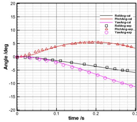
Figure 5 Variation of attitude angle of missile with time
