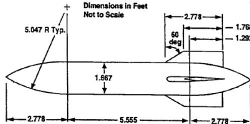
Figure 2 Geometric dimension of missile (unit: feet)
