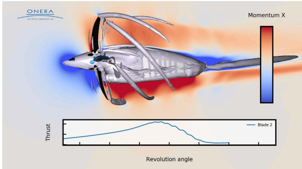
Figure 8 - Momentum field and Q-criterion of the complete configuration.
