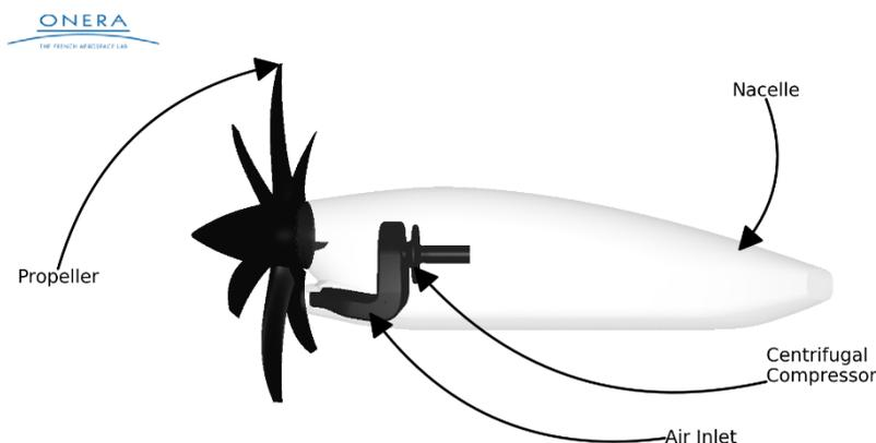
Figure 6 - Simulated configuration of the Tech TP demonstrator showing also the inside of the nacelle.
