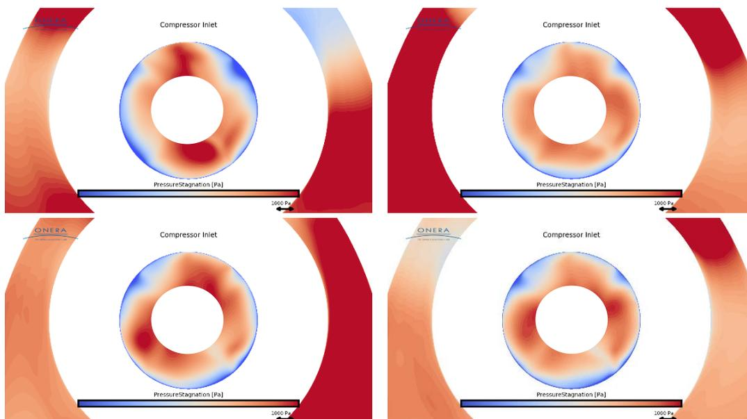
Figure 11 - Distortion in stagnation pressure at the compressor inlet at four different time instants (true inner radius of compressor not shown).
