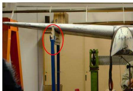
Figure 6 - Support of the half wing
