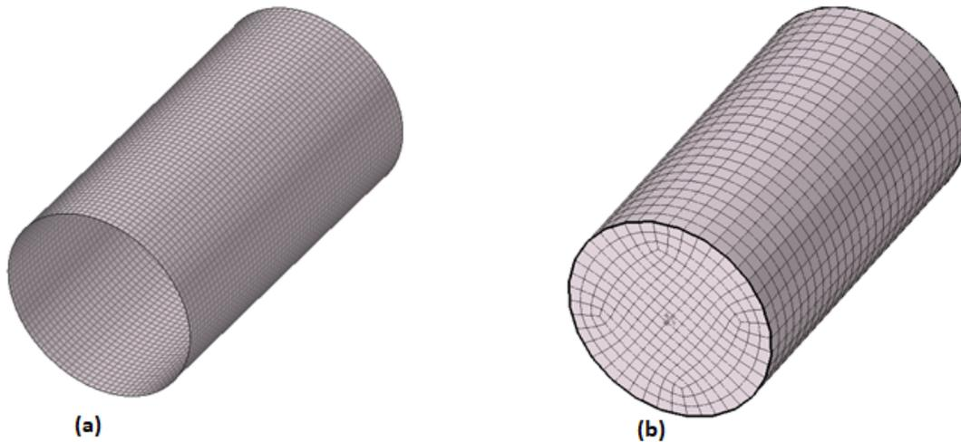
Figure 2 – The FEM geometry on which the natural mode are extracted. (a) Shell structure. (b) Cylindrical fluid cavity.
