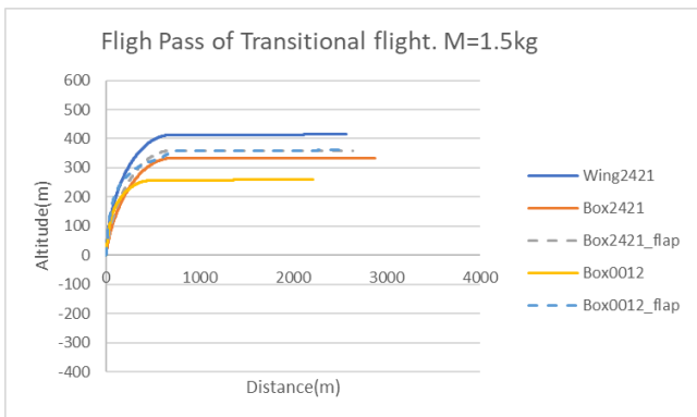
Figure 16 - Transitional flight path maintained at 8000RPM of each configuration with 1.5 kg aircraft(left) and 2.0 kg aircraft(right).
