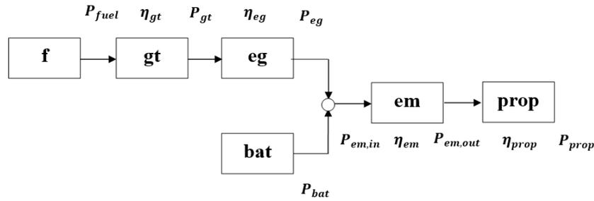
Figure 2: Schematic of the series hybrid-electric powerplant.
