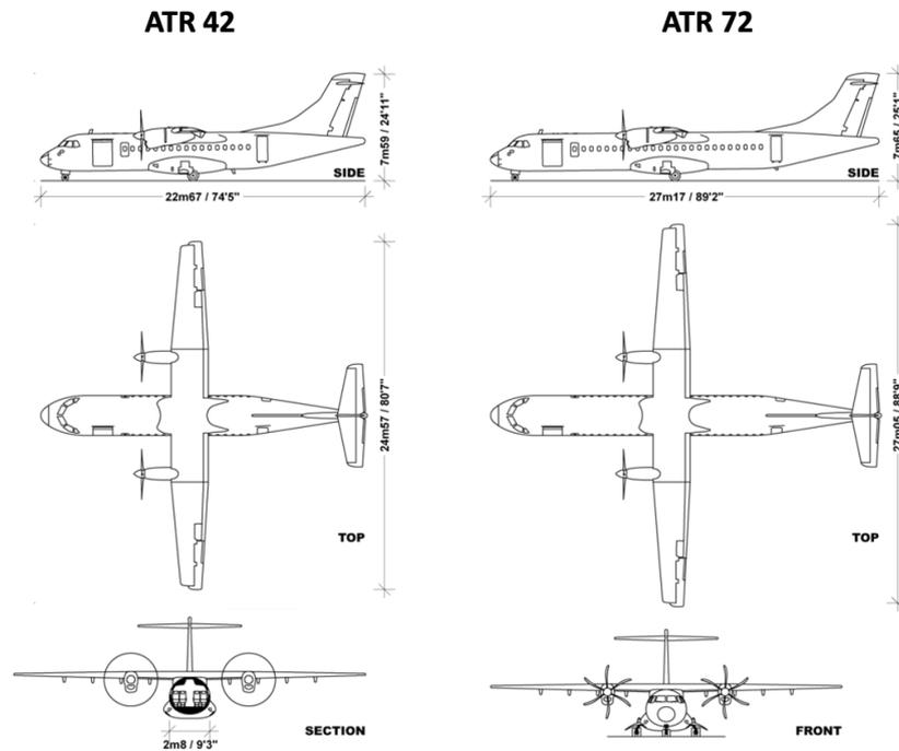
Figure 1. Schematic of the ATR 42 and ATR 72 respectively [12]
