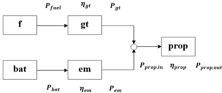
Figure 3: Schematic of the parallel hybrid-electric powerplant.
