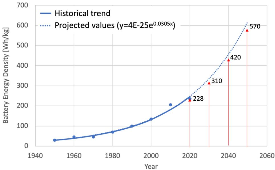
Figure 5: Energy density improvement in battery technology. Data extracted from [23]
