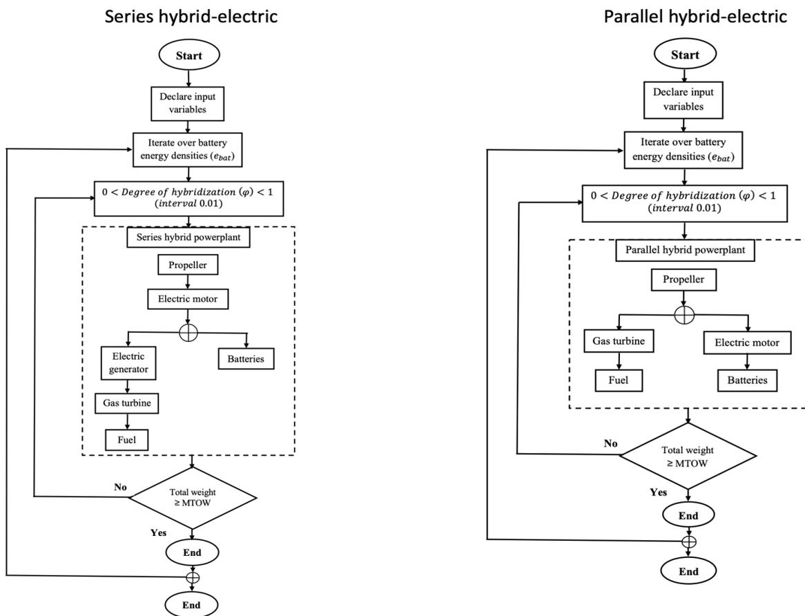
Figure 4: Schematic of the iterative model for the series hybrid-electric (left) and parallel hybrid-electric (right)
