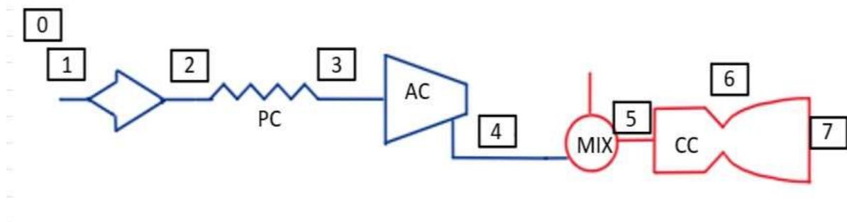
Figure 7 - Ramjet with precooler and compressor scheme.
