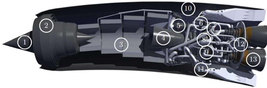
Figure 2 - From [5]: SABRE section: 1) movable spike 2) intake 3) precooler 4) air compressor 5) pre-burner and reheat (HX3) 6) helium circulator 7) H2 pump 8) He turbine and regenerator (HX4) 9) LOx pump 10) spill duct 11) ramjet burn
