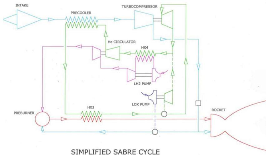
Figure 4 - SABRE cycle in both air breathing and rocket modes (from [6])
