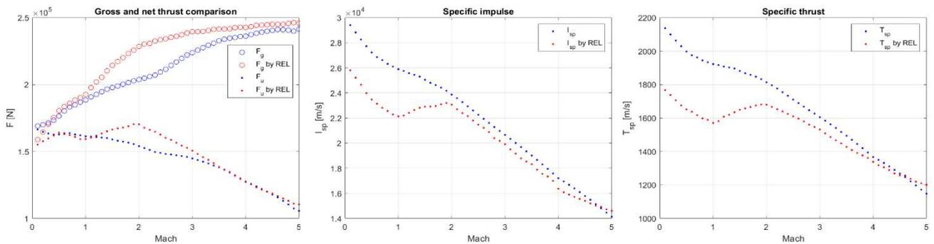
Figure 14 - Gross and uninstalled thrust, specific impulse and specific thrust comparison for the complete air cycle model.
