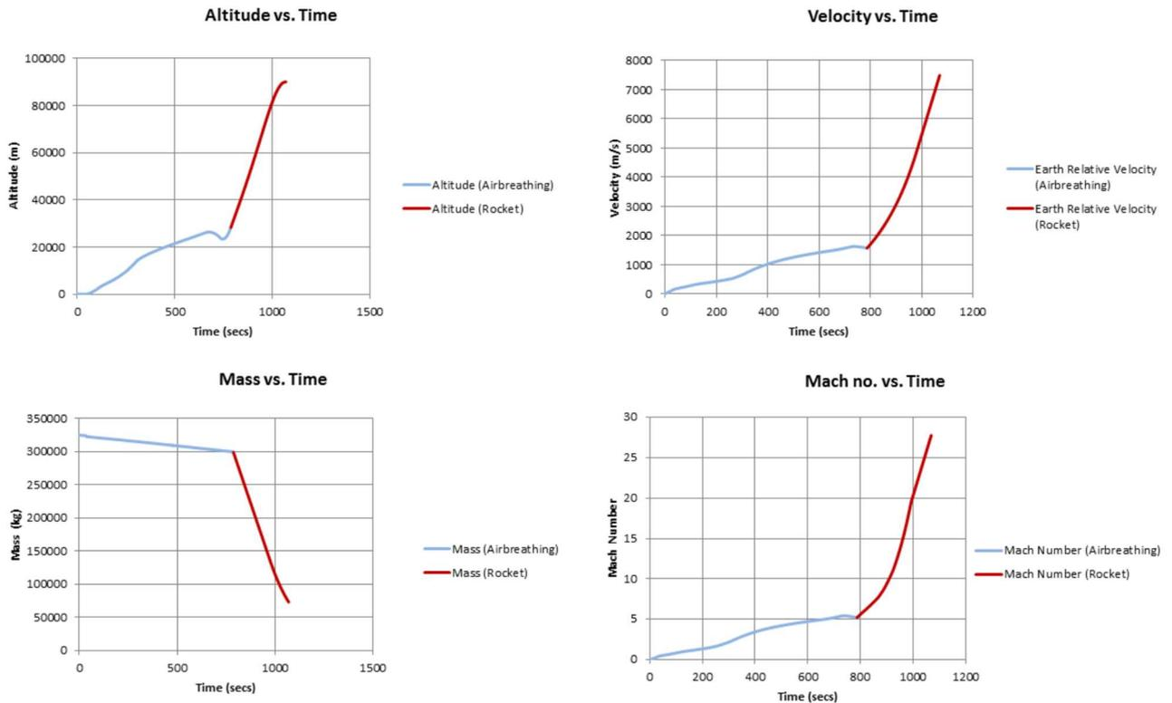
Figure 3 - trajectory of the typical mission of Skylon (from [3]).
