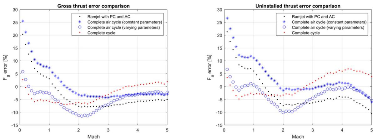
Figure 19 - Comparison of the errors of gross and net thrust of all the models.
