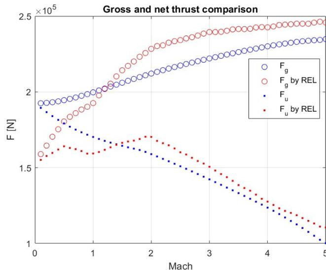
Figure 12 - Gross and uninstalled thrust comparison for the ramjet with precooler and compressor model.
