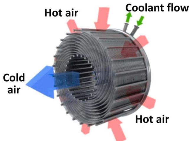
Figure 5 - Scheme of the SABRE precooler (from [9])
