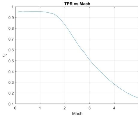
Figure 9 - total pressure recovery of the real intake along the trajectory.
