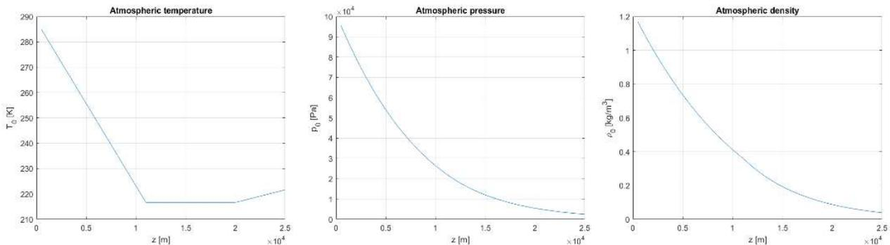
Figure 6 - Ambient characteristics at different altitude.
