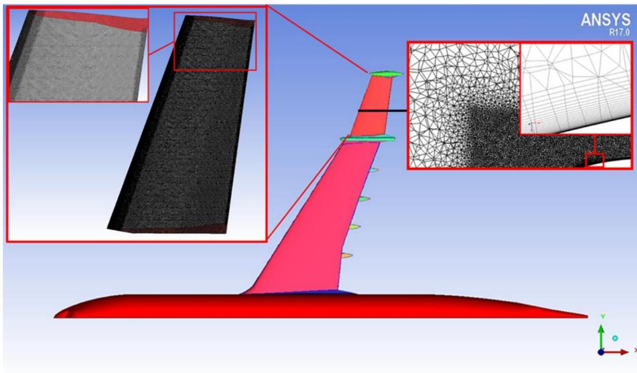
Figure 4 – Geometry provided by AIRBUS and parts of the mesh used for the CFD analysis.
