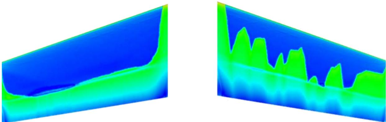
Figure 7 – Skin friction from CFD calculations based on transition line from flight test.
