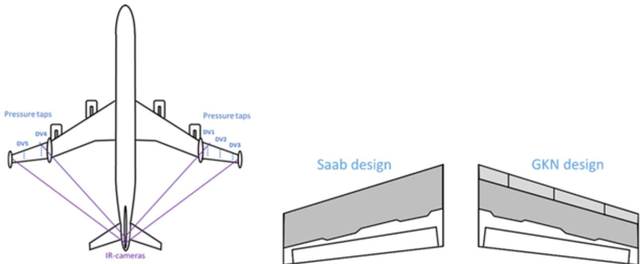
Figure 2 – The BLADE demonstrator aircraft with the different wing panel designs.
