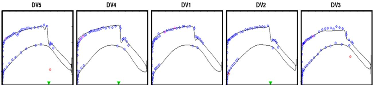
Figure 5 – Comparison of pressure coefficient from CFD calculations with flight test measurements.
