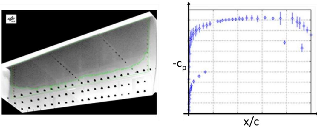
Figure 3 –IR data including a transition line (left, data from DLR) and pressure measurements including 95% confidence interval (right, data from AIRBUS).
