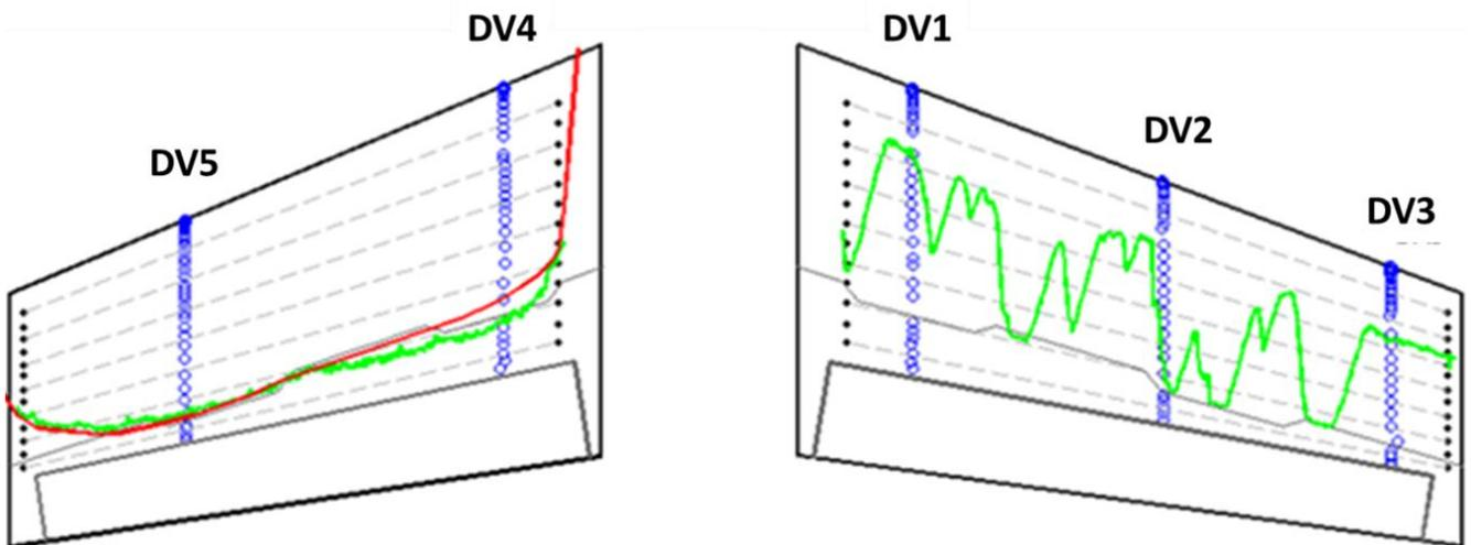
Figure 6 – Transition lines used for the CFD calculations based on flight-tested data, detected by DLR shown in green and some minor adjustments from Saab in red for the left wing panel.
