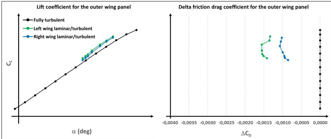
Figure 8 – Lift and delta frictional drag coefficients for the fully turbulent, left and right wing panel.
