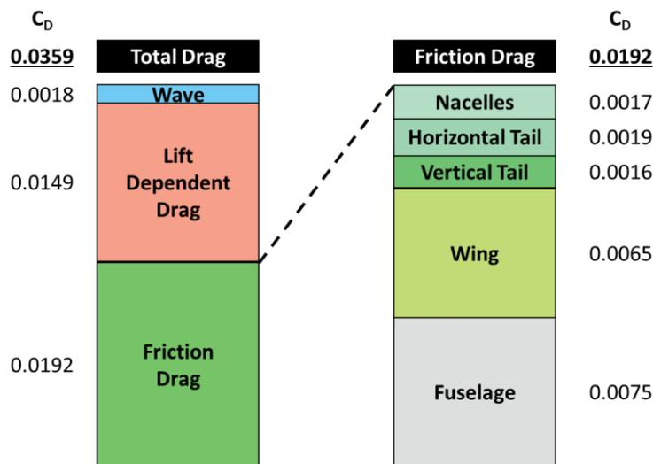
Figure 10 – Drag components of an A320 with a reduced wing sweep.
