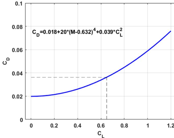
Figure 9 – A320 drag coefficient for M=0.73 with a model taken from [5]. The dashed line show  $C_D=0.0361$  for design  $C_L=0.65$ .
