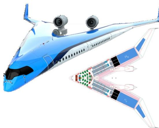
Figure 11: The Flying V concept with hydrogen propulsion (Ref: TU Delft, [6])
