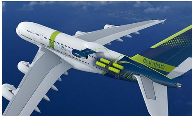
Figure 8: Airbus A380 Flying testbed for ZEROe Hydrogen propulsion architecture
