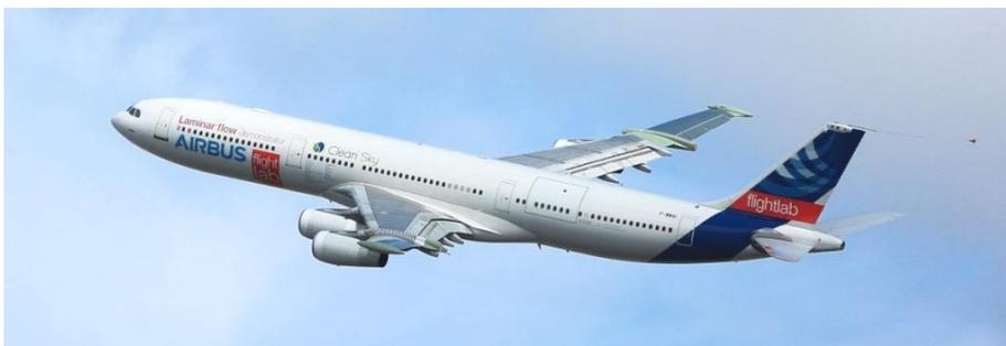
Figure 5: BLADE flight test demonstrator for natural laminar flow wing technology
