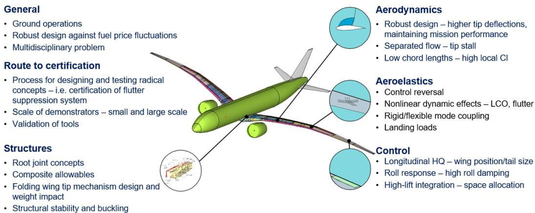
Figure 4: Technology challenges for the development of a high aspect ratio wing
