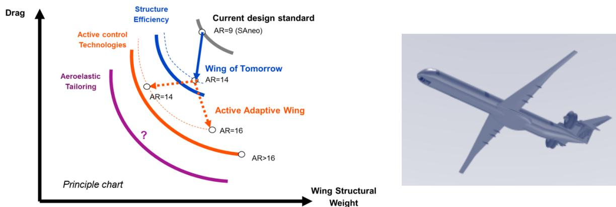
Figure 2: Increased aspect ratio to further optimize drag
