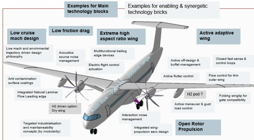
Figure 3: An ultraefficient aircraft concept
