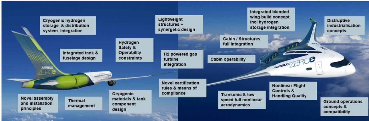
Figure 12: Selected examples on Airbus ZEROe concepts for Aircraft level design integration challenges of technology bricks, requiring a full multidisciplinary end-to-end modelling chain
