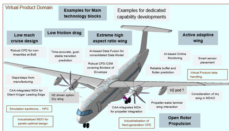
Figure 10: Next generation capabilities required to mature future technology on virtual product level (Picture shows examples related to the above-mentioned ultraefficient aircraft concept)
