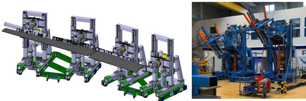
Figure 7: Modular testing bench for future Airbus wing-moveables design solutions
