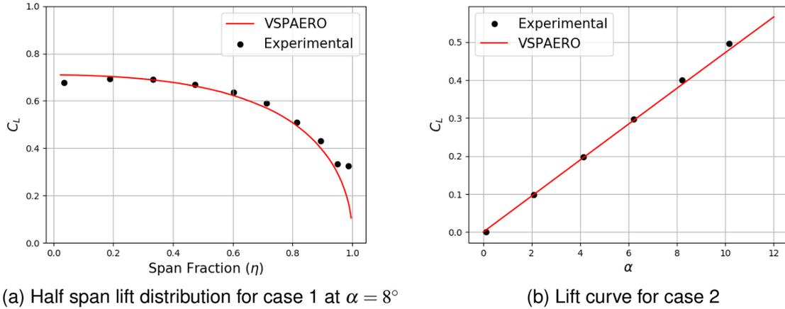
Figure 3 – Comparison between experimental results and VSPAERO for various wing cases
