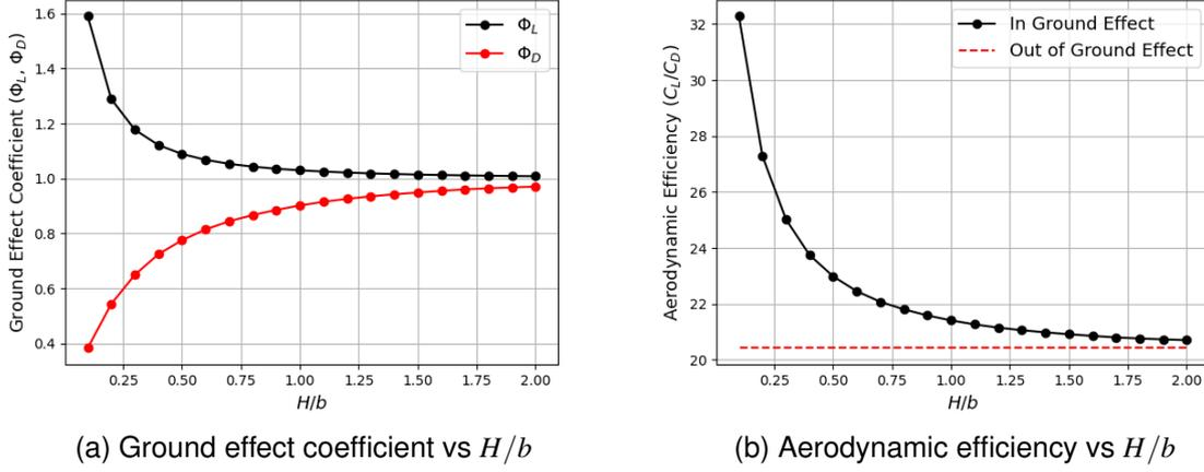
Figure 2 – Influence of ground effect coefficient and aerodynamic efficiency on ratio of distance from ground to wingspan ( $H/b$ ) for the baseline wing
