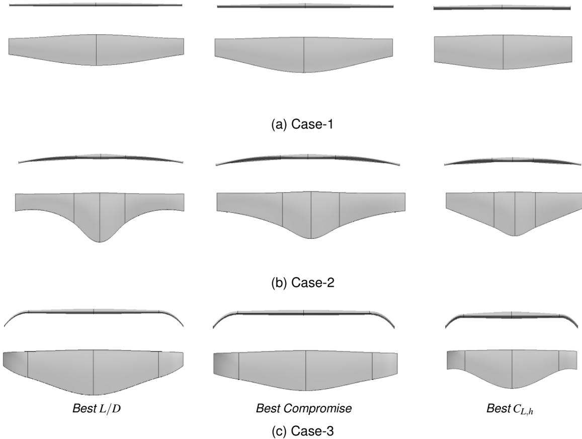
Figure 5 – Optimized planform shapes obtained from all the three cases. Left side shapes corresponds to best  $L/D$  ratio, right side shapes corresponds to best  $C_{L,h}$ , shapes in the middles corresponds to best compromise solution
