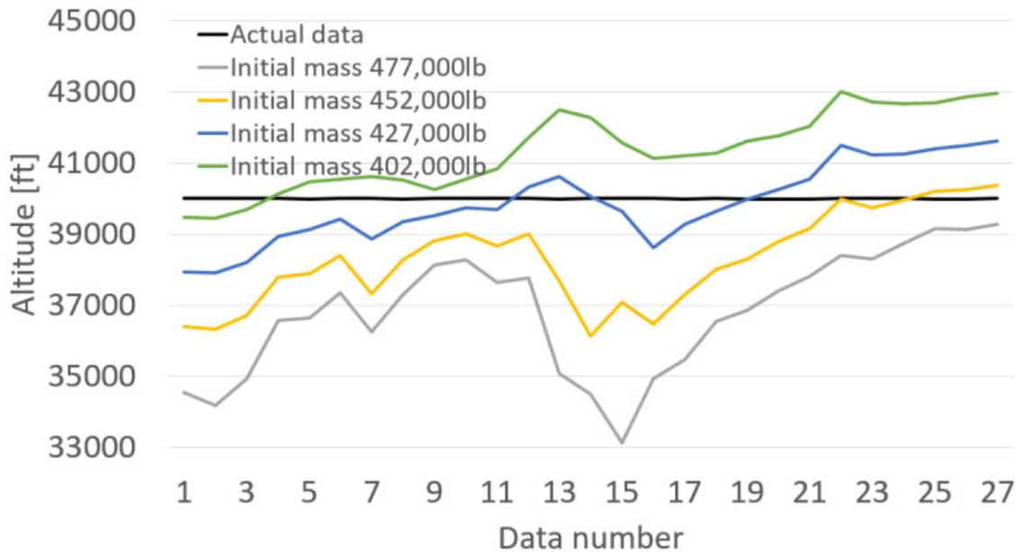
Figure 3 – Actual altitude and the cost-optimal altitude in each initial mass. (Flight ID: 4)
