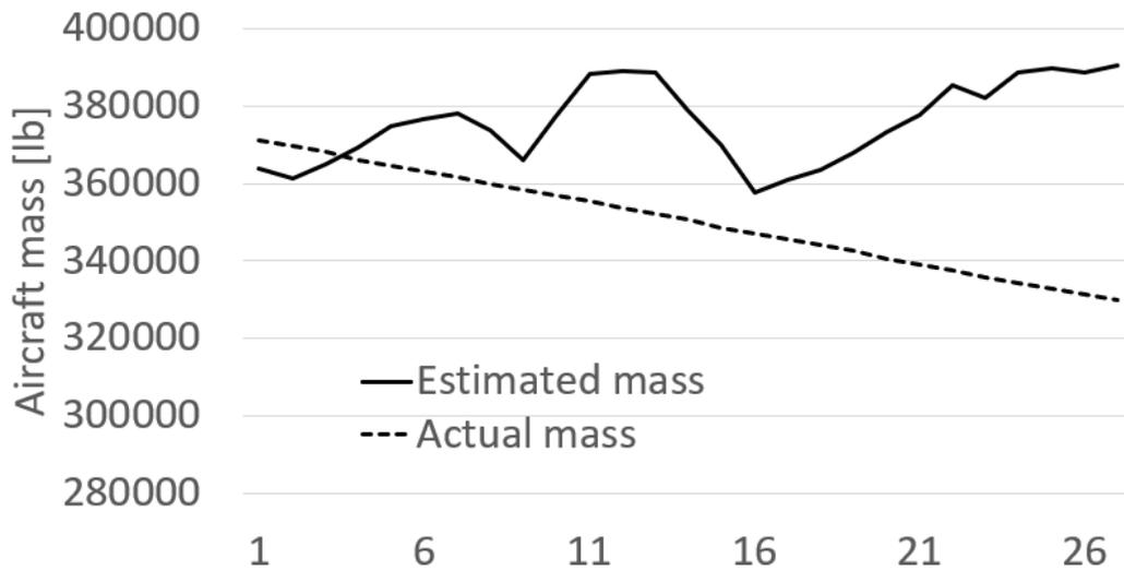
Figure 2 – Mass estimation on a single flight. (Flight ID: 4)
