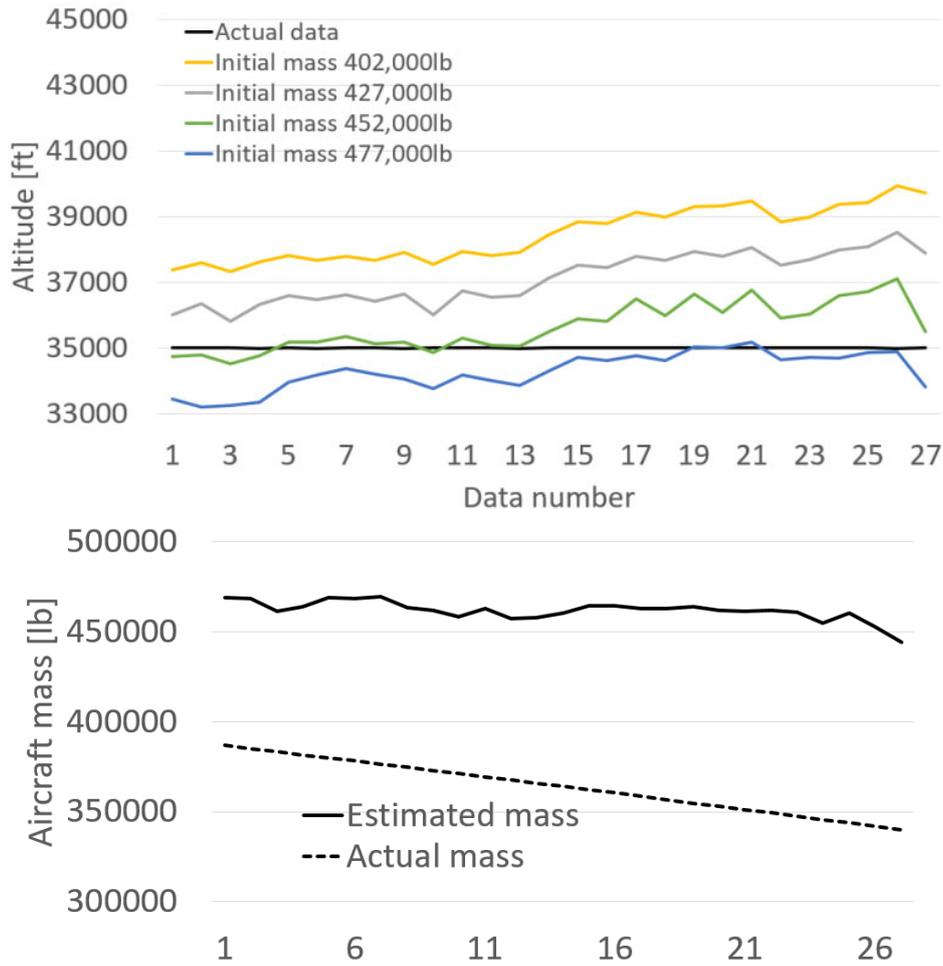
Figure 7 – The cost-optimal altitude and actual altitude, and the mass estimation result.
