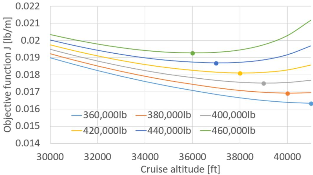
Figure 1 – The objective function vs. cruise altitude with various aircraft mass. (The dots indicate the optimal altitude in each aircraft mass.)
