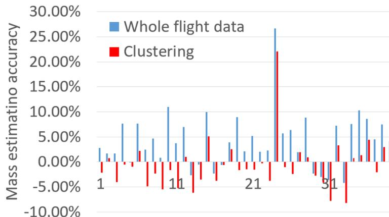
Figure 8 – Comparison of mass estimation error with usnig whole flight data and clustering method. (MAE = 3.29 % for clustering)
