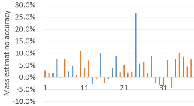
Figure 5 – Mass estimation with whole flight data. (MAE=5.23%) Orange bars indicate the flights where the cruise altitude changes within data samples.
