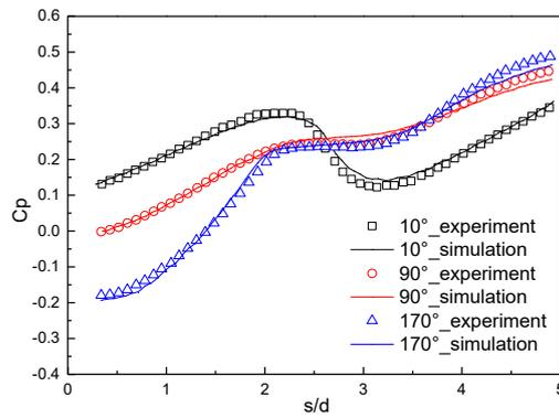
Figure 3 – Axial distribution of pressure coefficient
