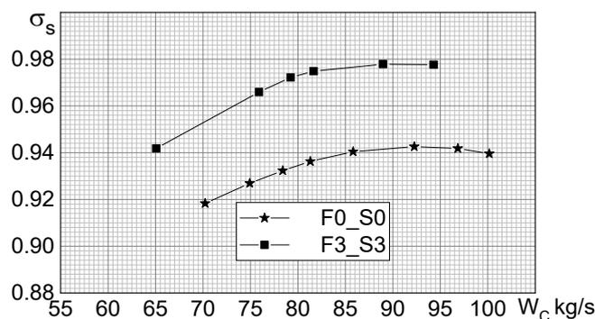
Figure 21 – Total pressure recovery coefficient for different parameter combinations
