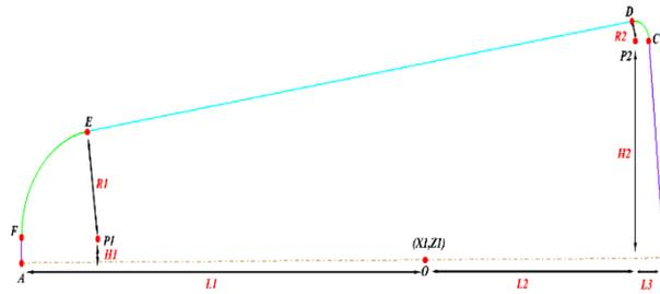
Figure 7 – Parametric shape of intake lip of submerged inlet
