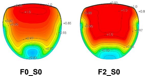
Figure 17 – Total pressure recovery coefficient counter of inlet cross section for different cases
