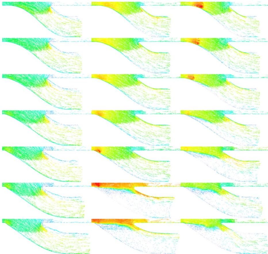
Figure 6 – Velocity vector diagram of different baseline inlet under different Mach numbers
