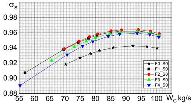
Figure 16 – Total pressure recovery coefficient for different flow direction design parameters
