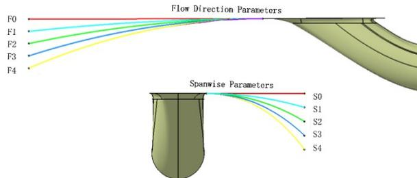
Figure 14 – Flow direction and spanwise design parameters
