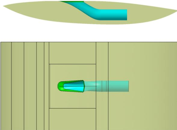
Figure 8 – The 3-D shape of submerged inlet
