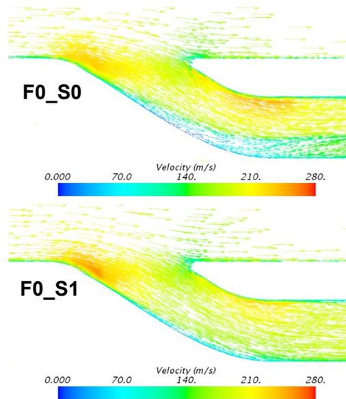
Figure 20 – Velocity vector distribution of inlet symmetrical plane for different cases (Ma=0.6)
