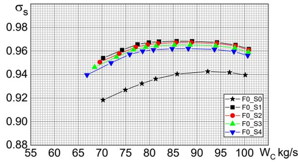
Figure 19 – Total pressure recovery coefficient for different span wise design parameters
