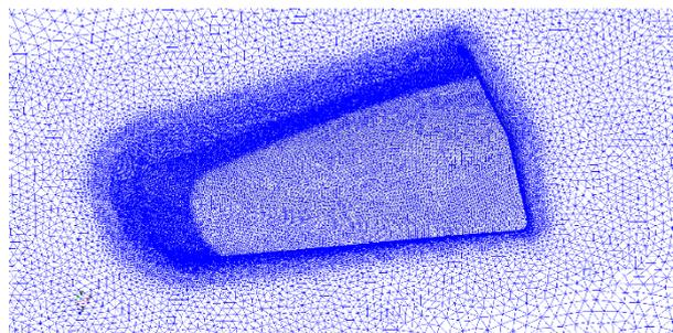
Figure 9 The surface mesh of the inlet
