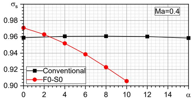
Figure 12 – The performances of different types of inlet under different angles of attack
