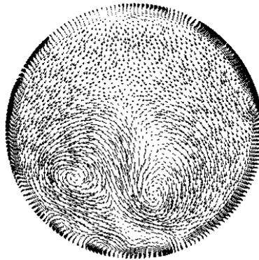
Figure 2 – Computed secondary flow in outlet cross section
