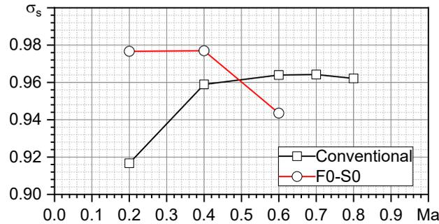
Figure 11 – The performances of different types of inlet under different Mach numbers
