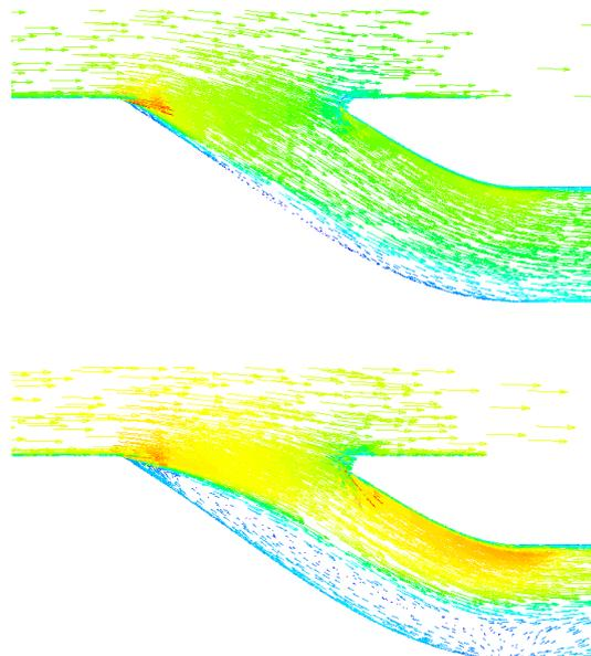
Figure 13 – Vector velocity of symmetric surface ( $Ma=0.6$ )
