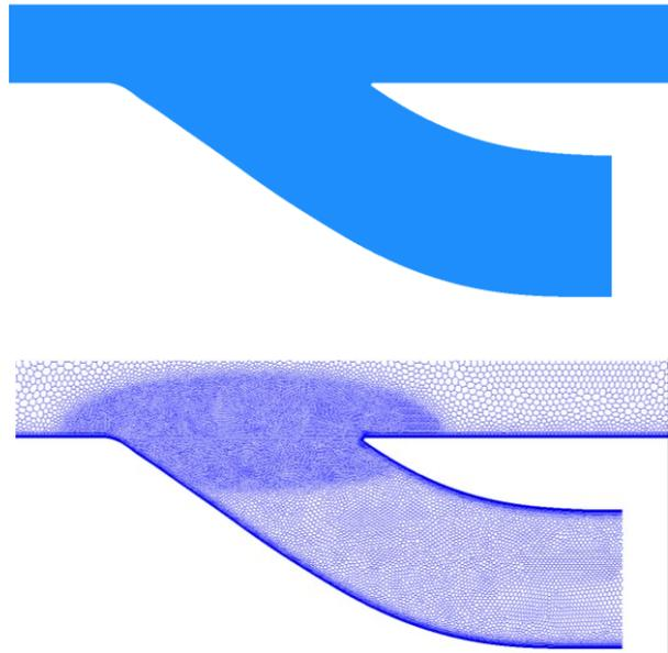
Figure 5 – The geometry and mesh of 2-D submerged inlet
