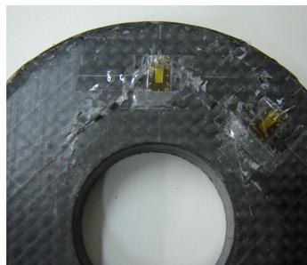
Figure 9 – Specimen with strain gauges attached on fracture region after the test.
