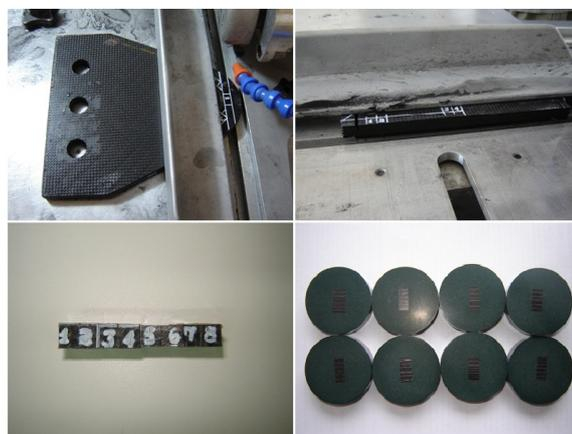
Figure 6 – Cut and preparation samples for analysis level of porosity and voids.
