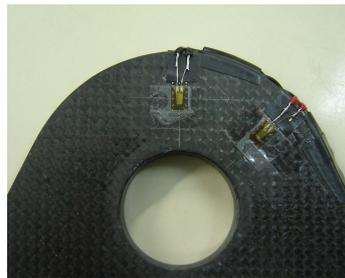
Figure 8 – Specimen with strain gauges attached before the test.
