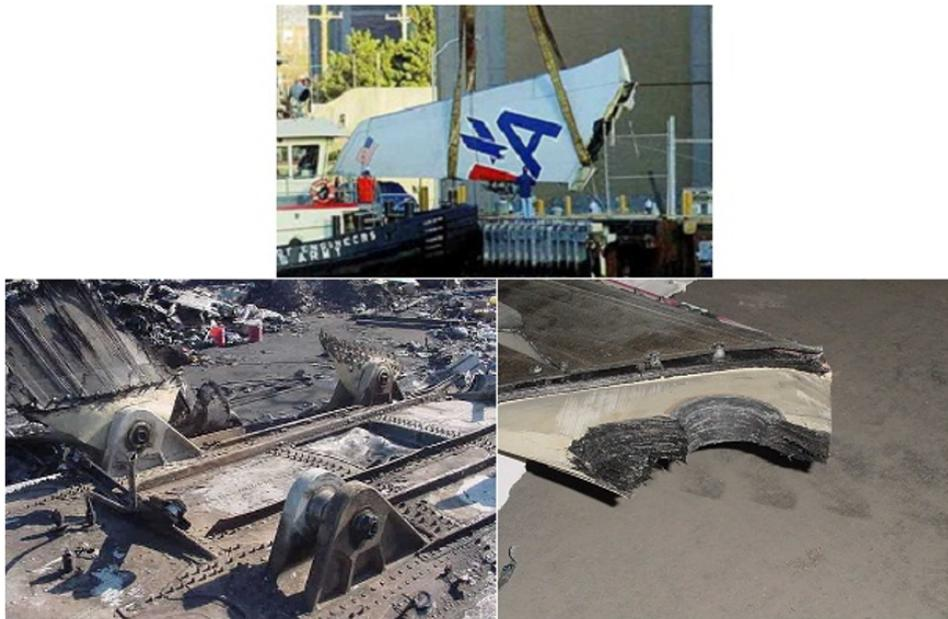
Figure 2 – Accident of AirBus A300-605R with lug failure manufactured by composite material.
