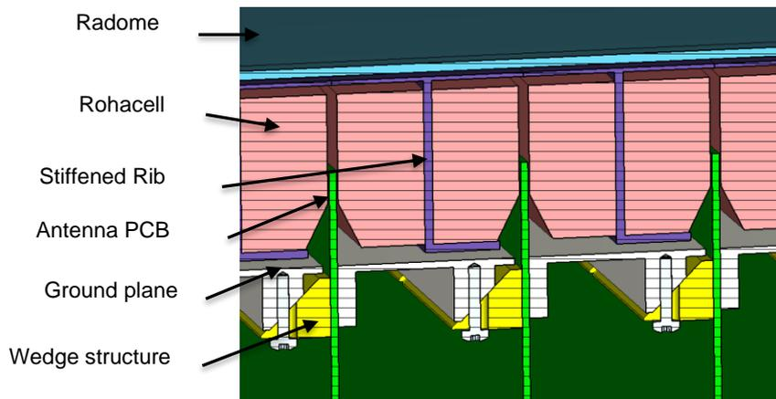
Figure 2 – Cross-section view of the antenna array
