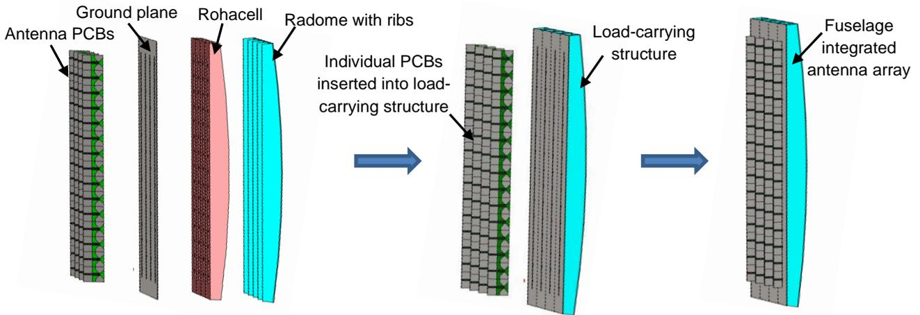
Figure 3 – Fuselage integrated antenna array and its assembly
