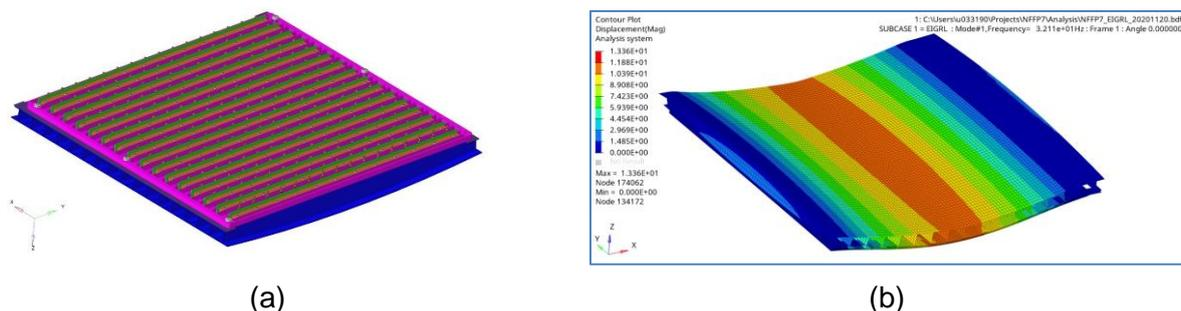
Figure 7 – FE-model and the mode shape. (a) FEM simulation model and (b) Lowest order eigenmode
