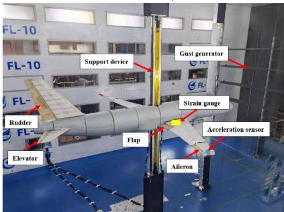
Figure 14 – Photo of gust load alleviation test
