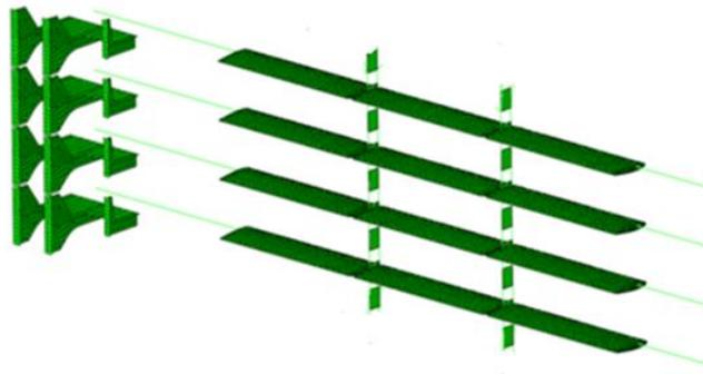
Figure 5 – Finite element model of generator
