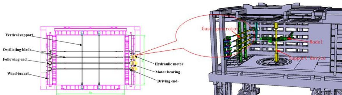
Figure 1 – Layout scheme of gust generator
