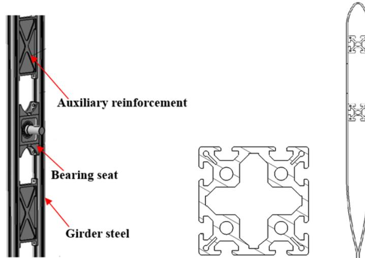
Figure 3 –Schematic diagram of vertical support structure
