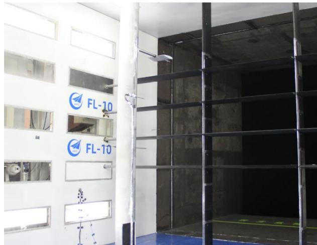
Figure 11 –Gust generator and flow field calibration device
