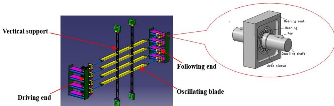
Figure 4 – Schematic diagram of the structure of the rotating shaft
