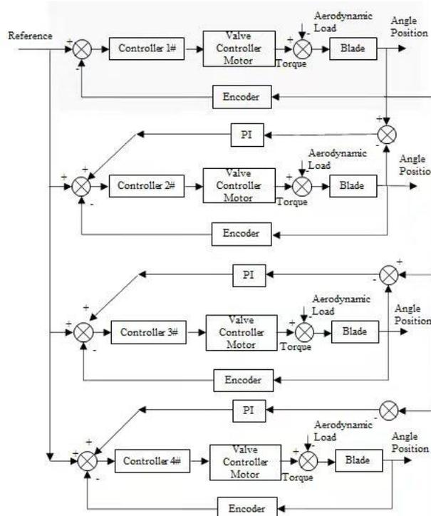
Figure 9 –The principle of synchronous control
