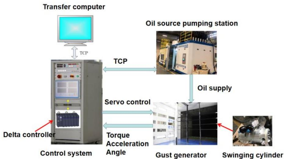
Figure 7 – Drive and control system of gust generator
