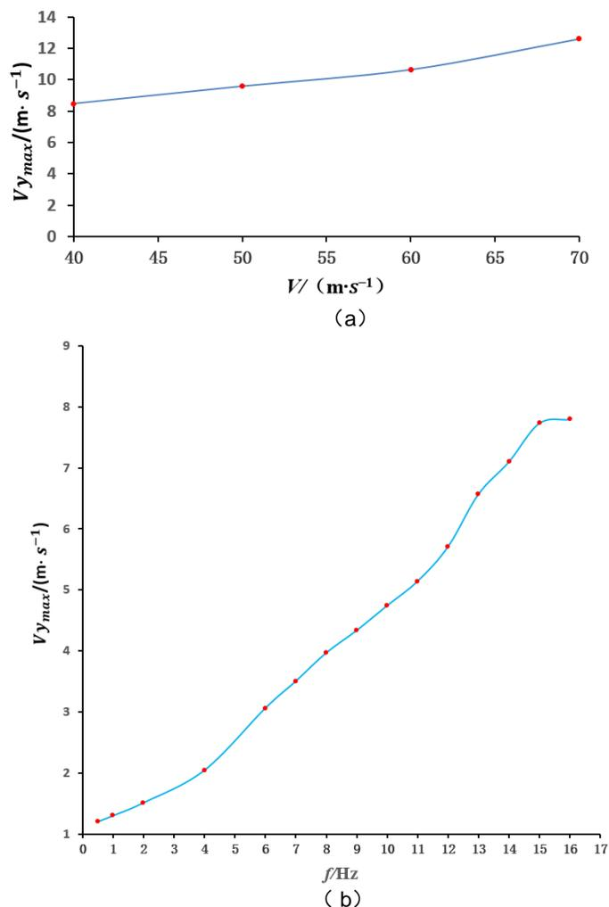
Figure 13 – Gust flow field curve (a) Variation of gust amplitude with incoming wind speed (b) Variation of gust amplitude with blade swing frequency
