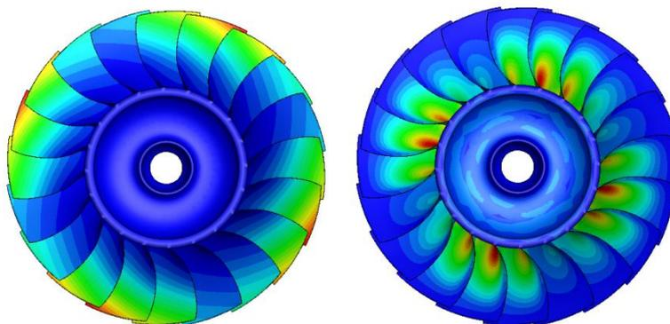
Figure 4–Relative von-mises stress distribution of the first bending mode at 2ND
