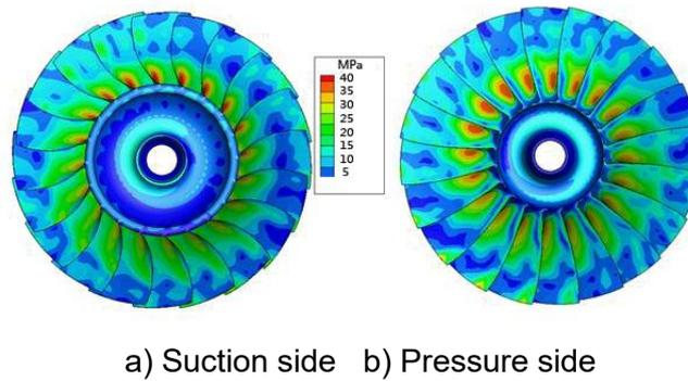
Figure 11-Dynamic stress results of the blade with asymmetry stator design
