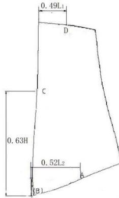
Figure9-Strain gauges mounted on the blade
