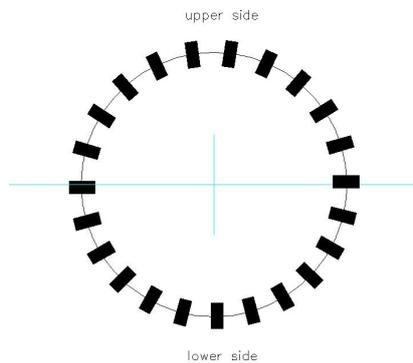
Figure10-Asymmetry stator design
