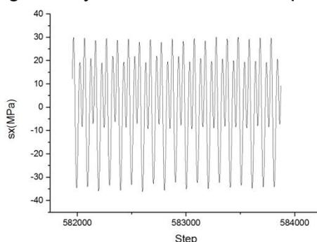
Figure7-Dynamic stress curve for first bending mode
