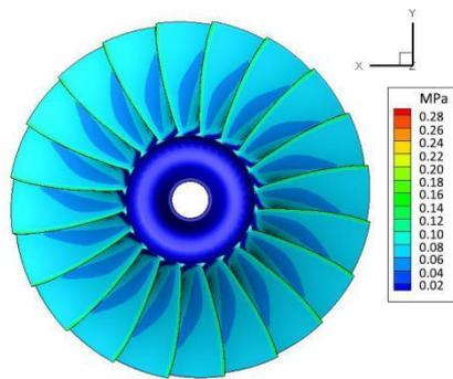
Figure5-Static pressure distribution after convergence
