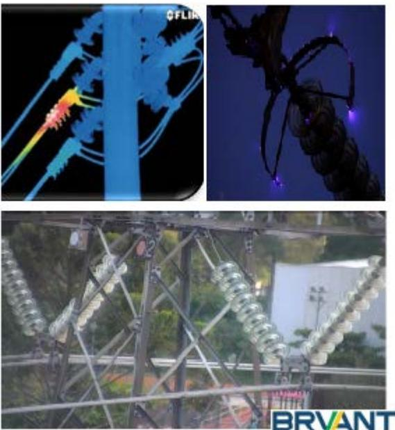
Figure 4 - Thermal, (2) Corona effect & (3) RGB (visible)
