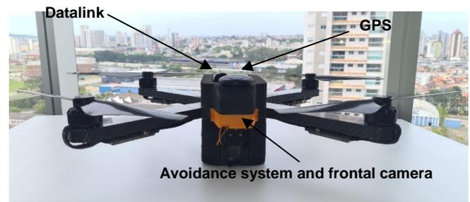
Figure 2 - BRV-03, Electric UAV prototype.
