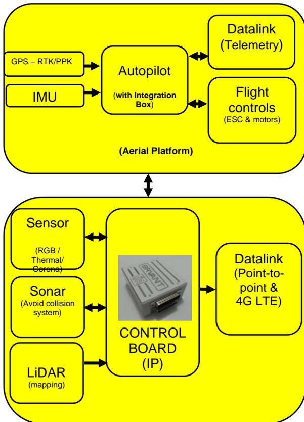
Figure 3 - The onboard equipment integration diagram.
