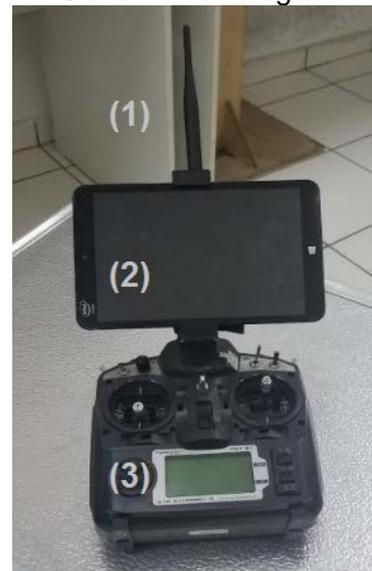
Figure 15 - Portable Command and Control Station (PCCS).
