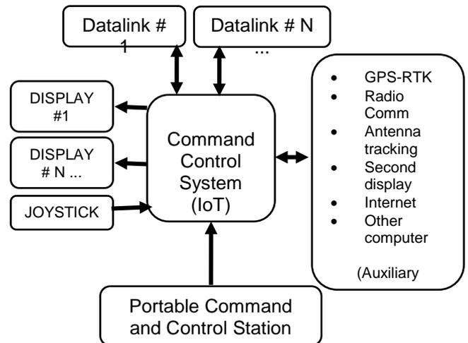
Figure 14 - Portable Command and Control Station block diagram.
