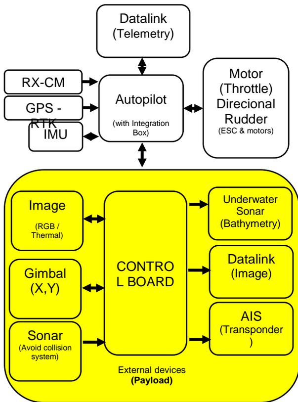
Figure 8 - Boat: The onboard equipment integration diagram.
