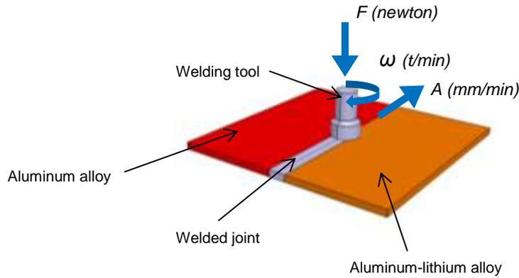
Figure 4 – Welding configuration.
