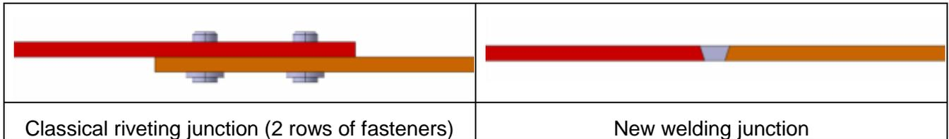
Figure 1 – Comparison riveting and welding junctions.
