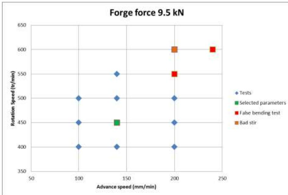
Figure 5 – Welding parameters.
