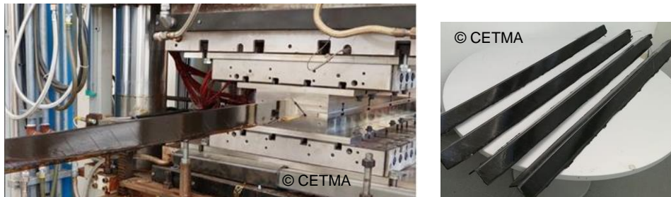
Figure 7 - L-stringer molded using Continuous Compression Molding, Courtesy of CETMA, CleanSky2 KEELBEMAN project [18]
