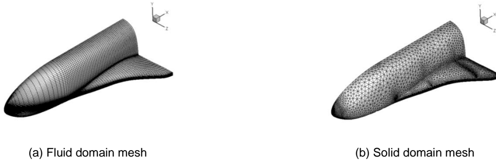
Figure 11 - Mesh of the Wing-body combination aircraft configuration
