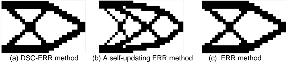
Figure 4.5 – Topology optimization of a cantilever beam by different methods
