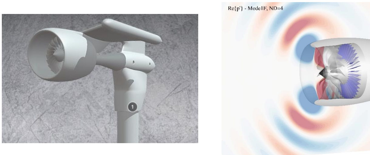
Figure 19 - SA²FIR Installation Rig from Clean Sky Initiative LPA 1 (left) and intake acoustic resonance flutter sensitivity study exploiting the test rig taken from [29]
