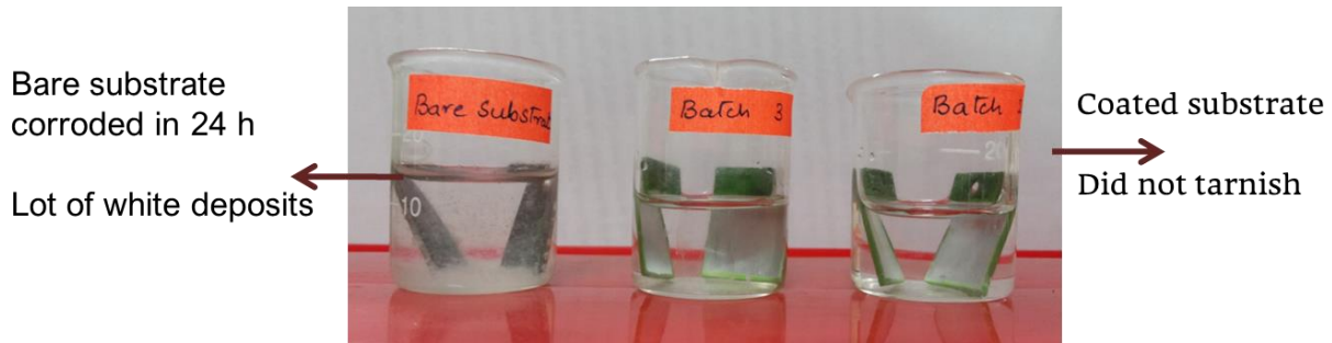
Figure 3 – Photograph of silica-alumina coatings with varied GPTMS and ASB mole ratio, immersed in NaCl solution
