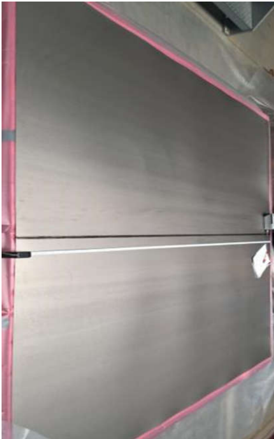
Oversize panel manufactured by welding performed by RJ-Lasertechnik
