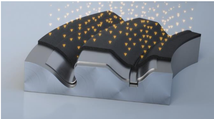
Figure 3 – The principle of the Quintus Flexform process
