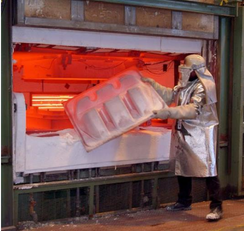
Figure 2 – Example of the traditional hot forming process
