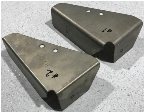
Figure 22 – Tool compensation for material spring back
