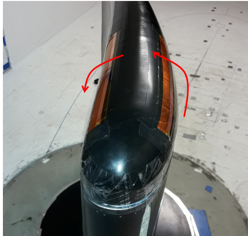
Figure 7 – DBD-PAs connected in parallel, the arrows illustrate the direction of the jets produced.
