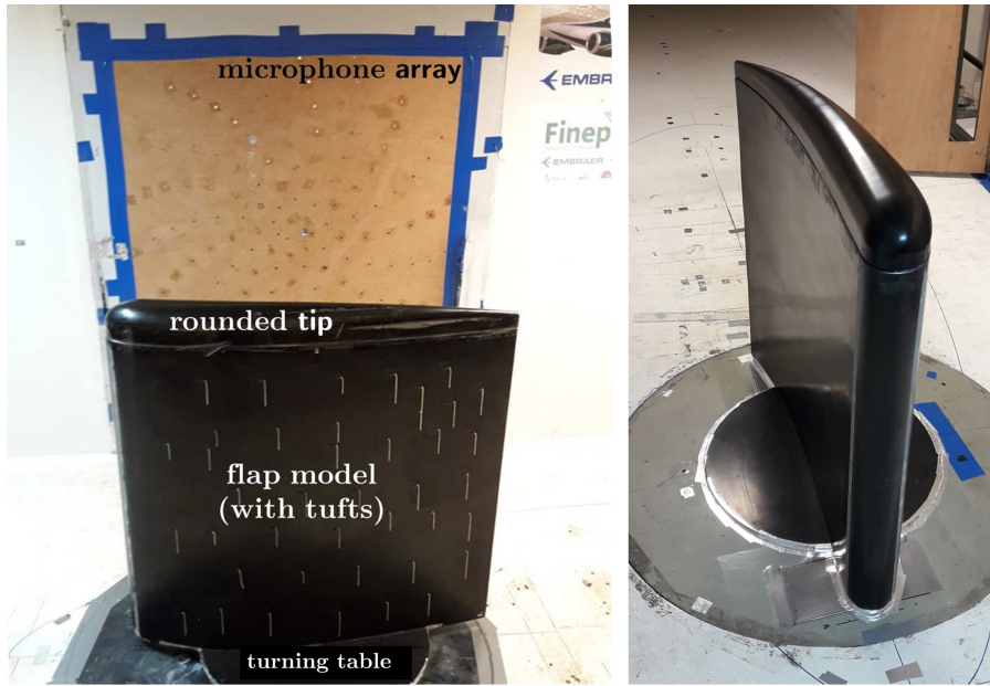
Figure 6 – Flap model installed at the test section of the LAE-1 wind tunnel.
