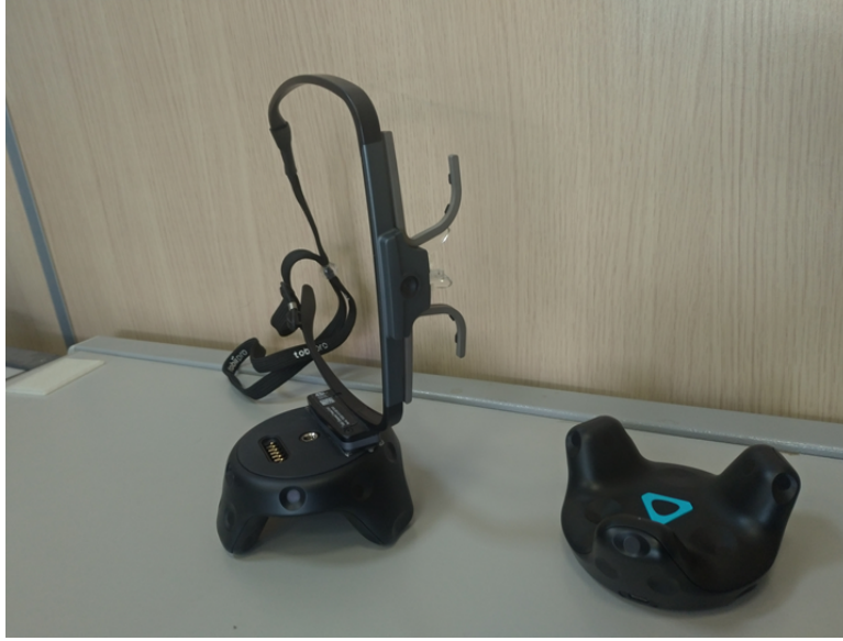
Figure 2 – The Wearable hardware used in the proposed system, a Tobii Pro Glasses 2 headset with an attached HTC Tracker.
