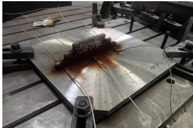
Fig. 7. Step component after printing.
