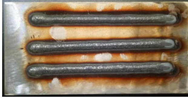
Fig. 3. Three weld beads for use in the heat source parameter calibration experiment.
