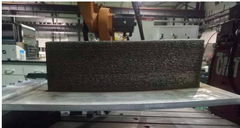
Fig. 12. Wall structure after printing.
