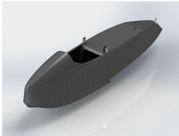
Figure 6 - Hull and attacks with the aircraft's wing plane
