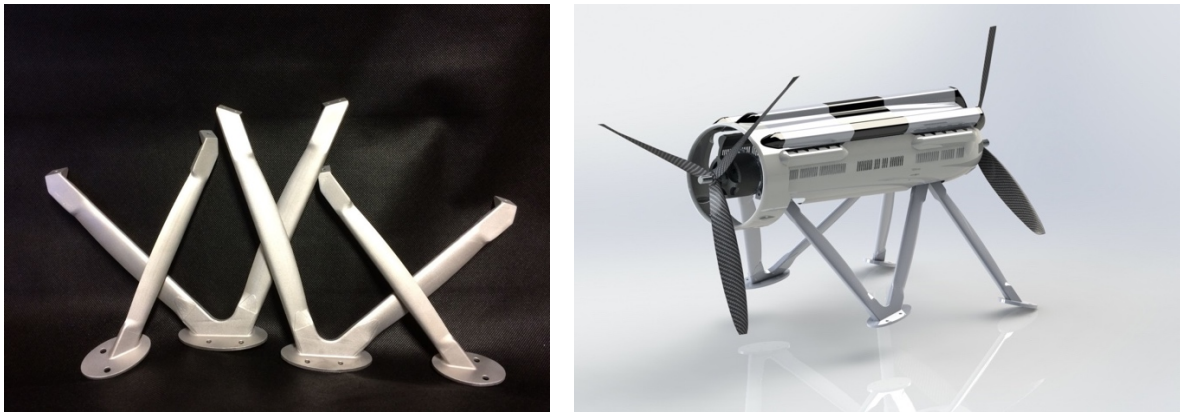
Figure 8 - Legs of the engine mount made of AM (left), CAD of the engine mount with fairing (right)
