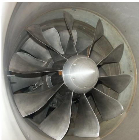
Figure 1 – Ducted counter-rotating fan model CRTF2A – front view.
