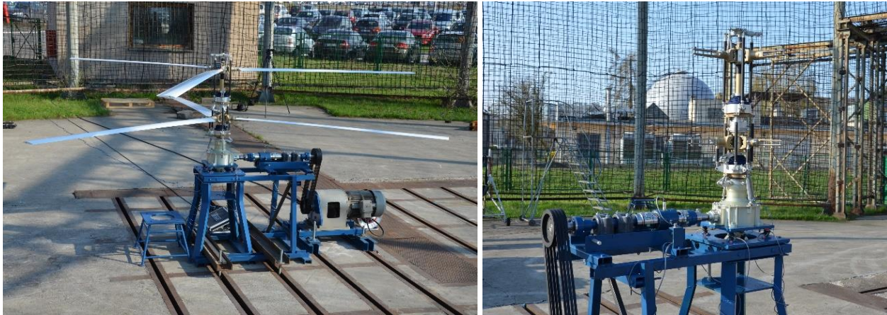
Figure 6 – Coaxial rotor whirl tower test stand [1].
