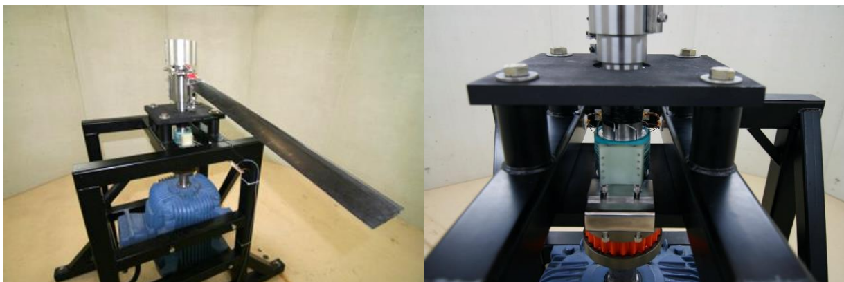
Figure 7 – The Whirl Tower Test Chamber and Test Stand [7]
