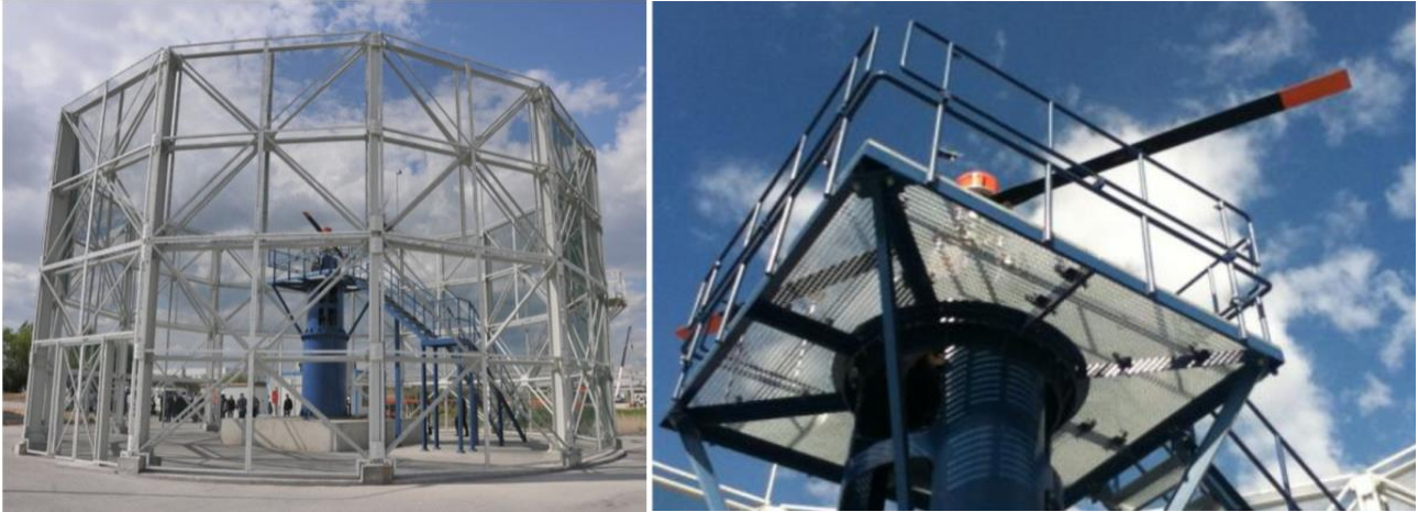
Figure 3 – The TAI whirl tower system [5].
