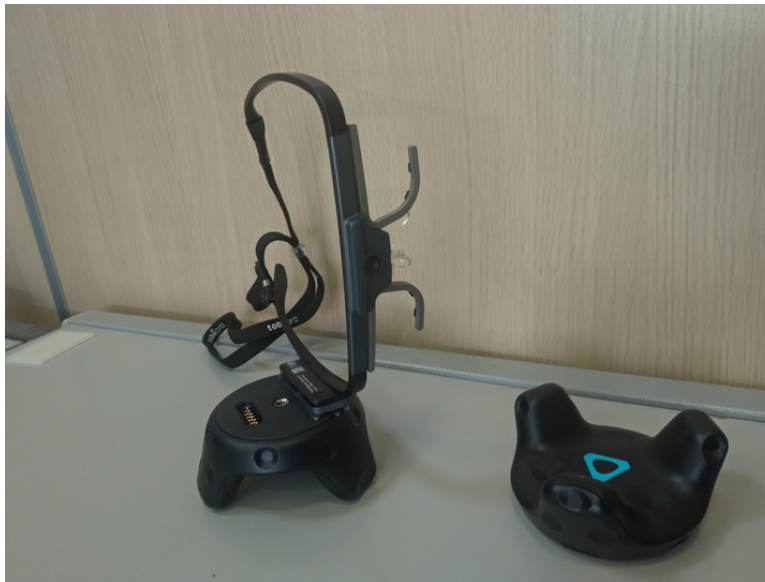
Figure 1 – The Wearable hardware used in the proposed system, a Tobii Pro Glasses 2 headset with an attached HTC Tracker.
