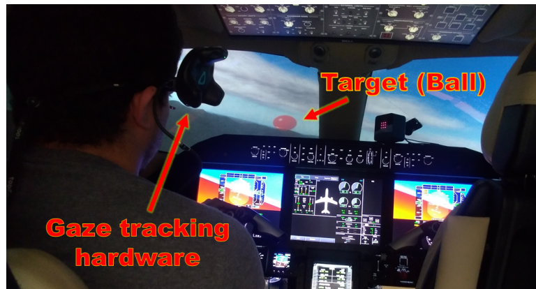
Figure 5 – A Test subject in SIVOR guiding the aircraft to the target using gaze.
