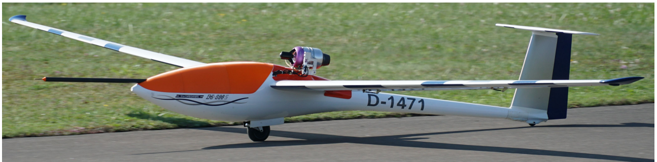
Figure 1 – Instrumented UAV CARF-Models Ltd. DG-800 S on the runway (picture courtesy of Lars H. Nagel).
