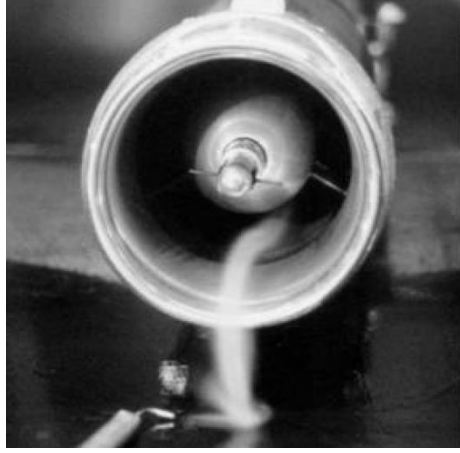
Figure 1 – Ground effect vortex observed in a wind tunnel model experiment [5]
