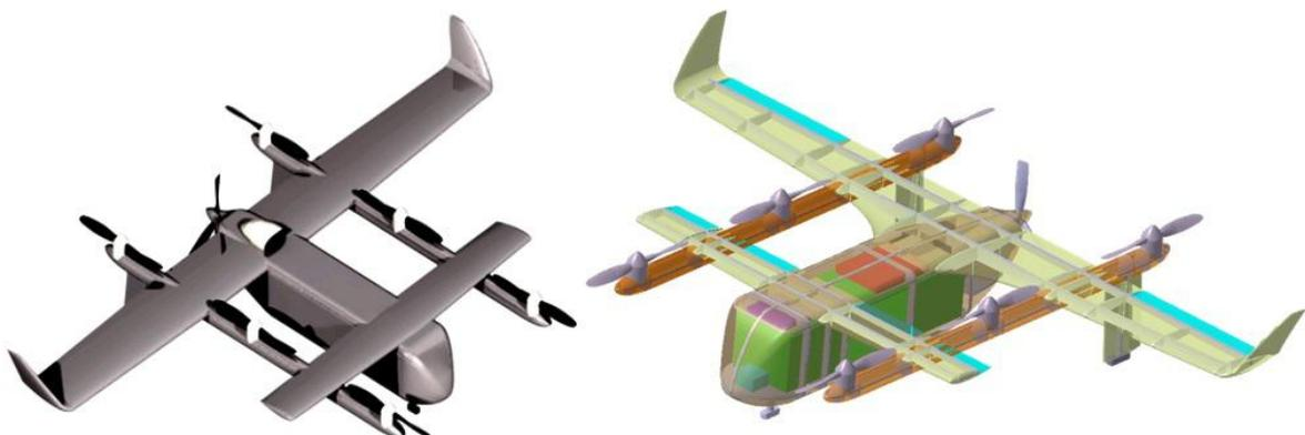
Figure 5 – Hybrid VTOL logistics UAV system
