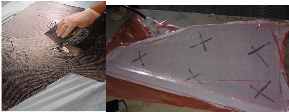
Figure 5: upper wing skin - hand layup and vacuum bag
