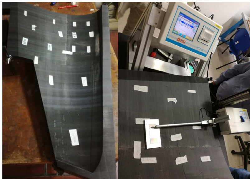
Figure 3: upper wing mould assembled and ready for roughness measurements.
