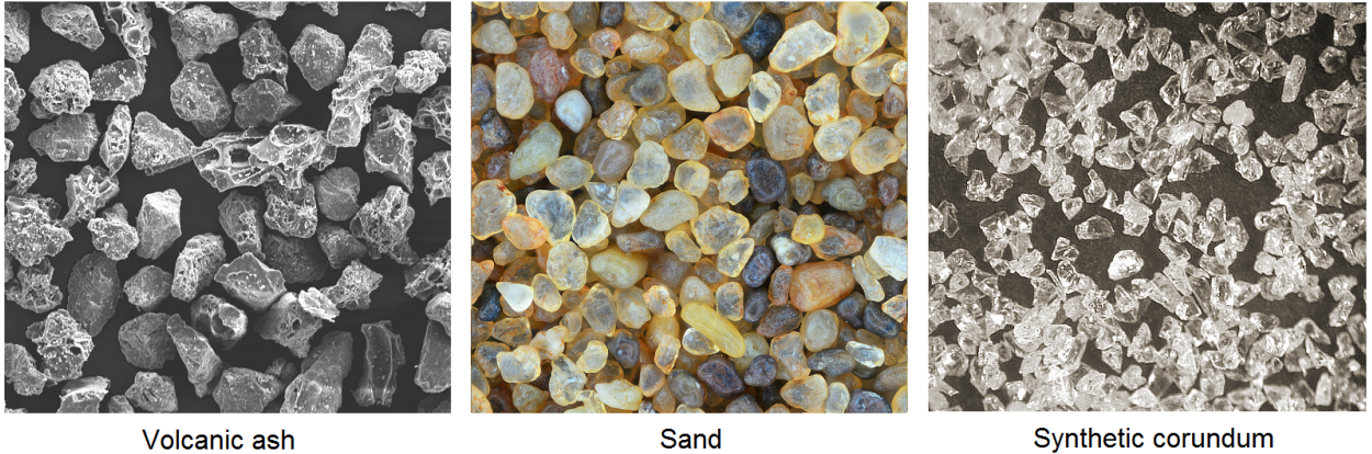
Figure 1 – Shape of natural and manufactured particles.
