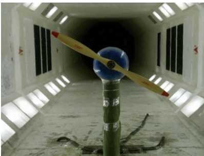
Figure 5 – Model of 1.2m diameter propeller (NF-3 wind tunnel of Northwestern Polytechnical University)
